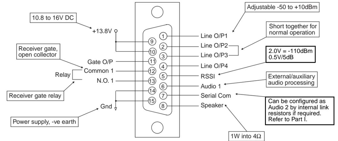
**Figure 1.3 T855 D-Range 1 Wiring - Rear View**
