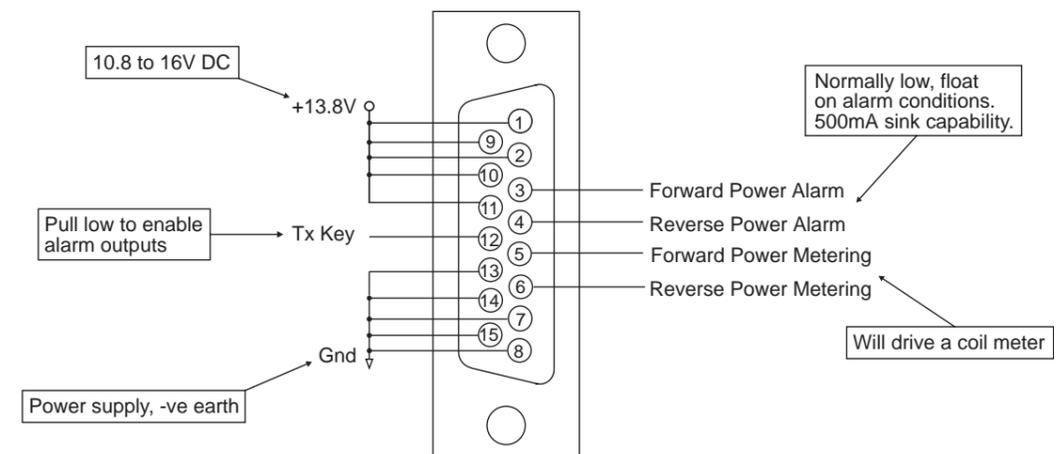
Figure 3.4 T858/859 D-Range Wiring - Rear View
