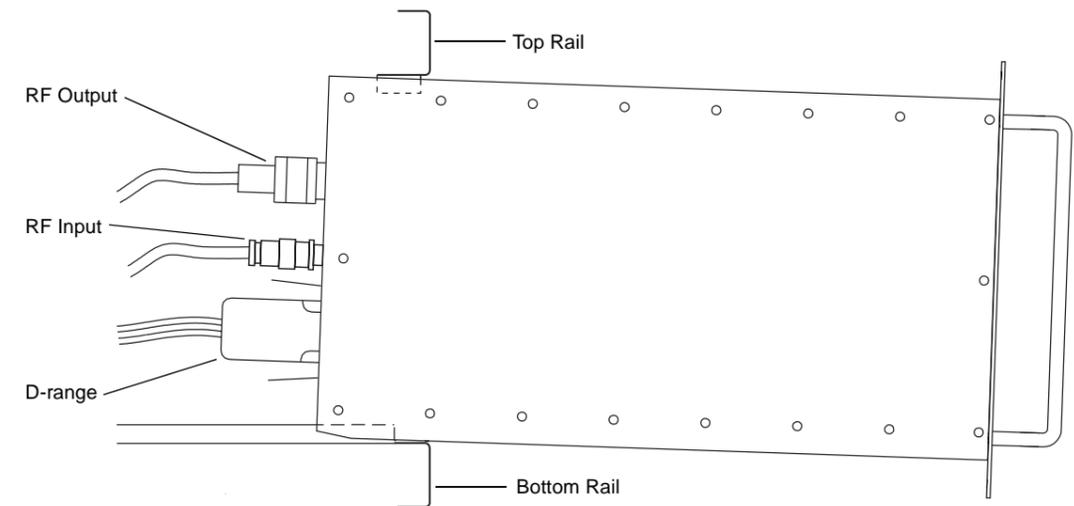
Figure 3.3 T858/859 PA In Latched Position
