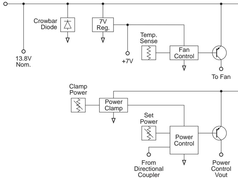
**Figure 2.4 T889 Power Supply & Regulator Circuitry Block Diagram**
