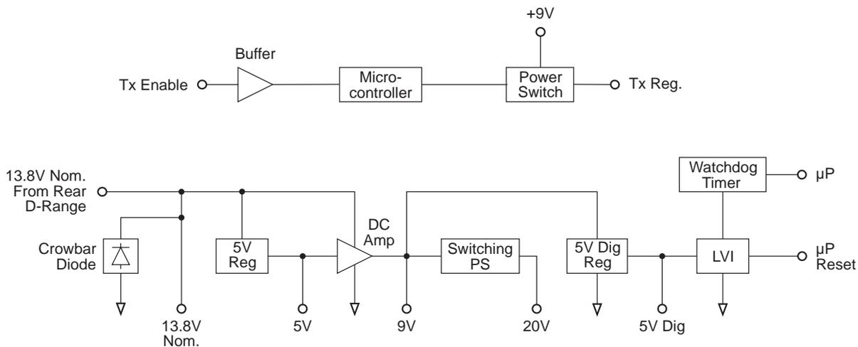
**Figure 2.5** T837 Power Supply & Regulators Block Diagram
