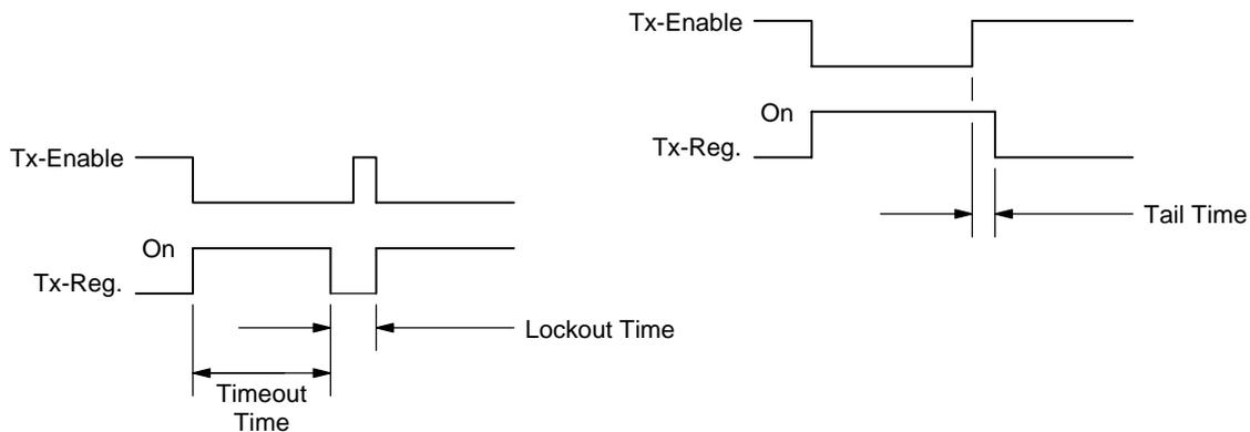
Figure 2.6 T837 Transmit Timers
