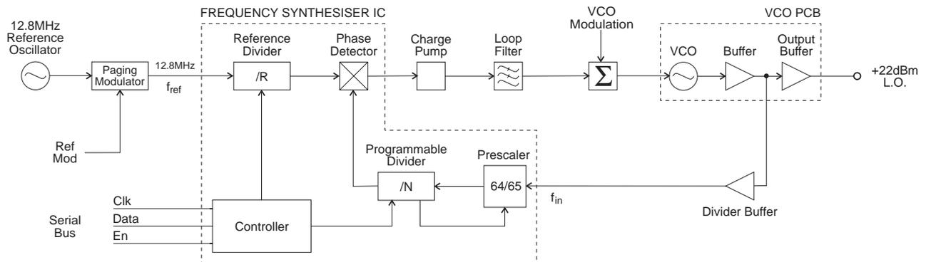
**Figure 2.3 T837 Synthesiser Block Diagram**
