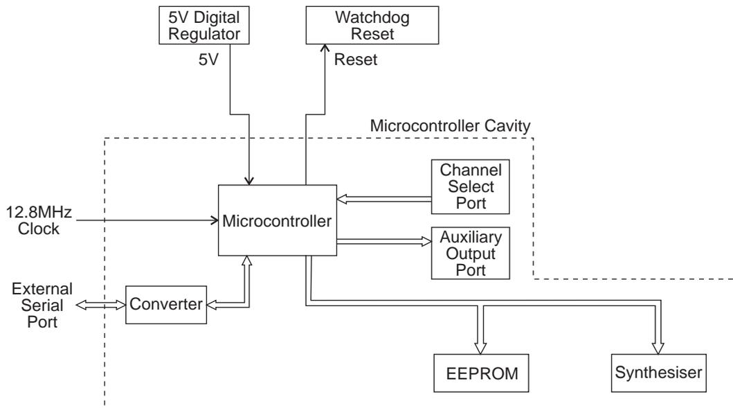
**Figure 2.2 T837 Microcontroller Block Diagram**
