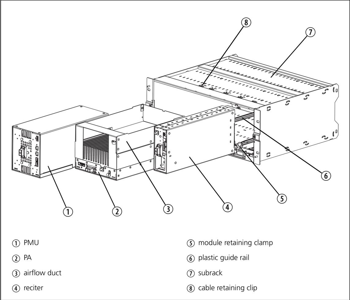
Figure 1.3 above shows the configuration for a typical single 100 W base station. The PMU occupies its normal slot at the left end of the subrack, with the PA directly beside it. The single reciter occupies the slot immediately to the right of the PA.
