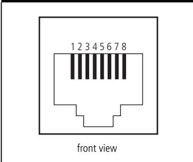
The diagram shows a front view of an 8-pin RJ45 socket. The pins are numbered 1 through 8 from left to right. Pin 5 is the tallest, pin 6 is the shortest, and pins 1, 2, 3, 4, 7, and 8 are of intermediate height. The label 'front view' is centered below the socket diagram.
