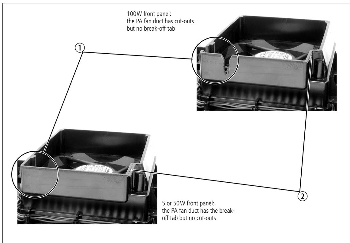
1. Before fitting the front panel, ensure that all cables are secured and positioned correctly so they are clear of the fan ducts (refer to [Figure 6.1 on page 55](#) and [Figure 6.2 on page 56](#)). Otherwise the panel may not fit properly, or you may damage the cables.
