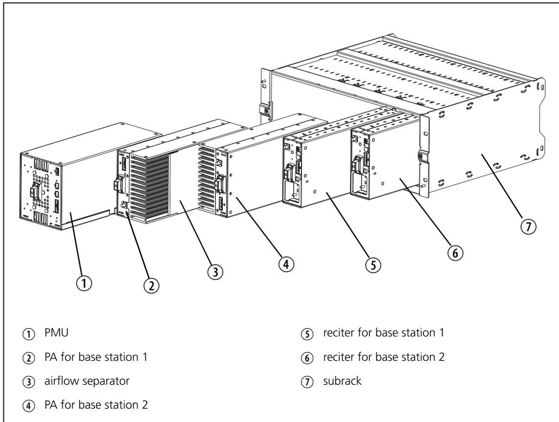
Figure 1.2 above shows the configuration for a typical dual 5 or 50W base station. The PMU occupies its normal slot at the left end of the subrack, with the reciters in the two right-hand slots.
