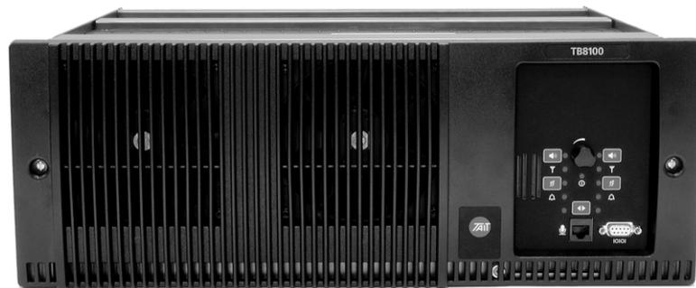
The TB8100 is a software-controlled base station system (BSS) which is designed for operation on most standard frequency ranges<sup>1</sup>. It makes extensive use of digital and DSP technology. Many operating parameters such as channel spacing, audio bandwidth, signalling, etc. are controlled by software. It is also capable of generating alarms for remote monitoring.
