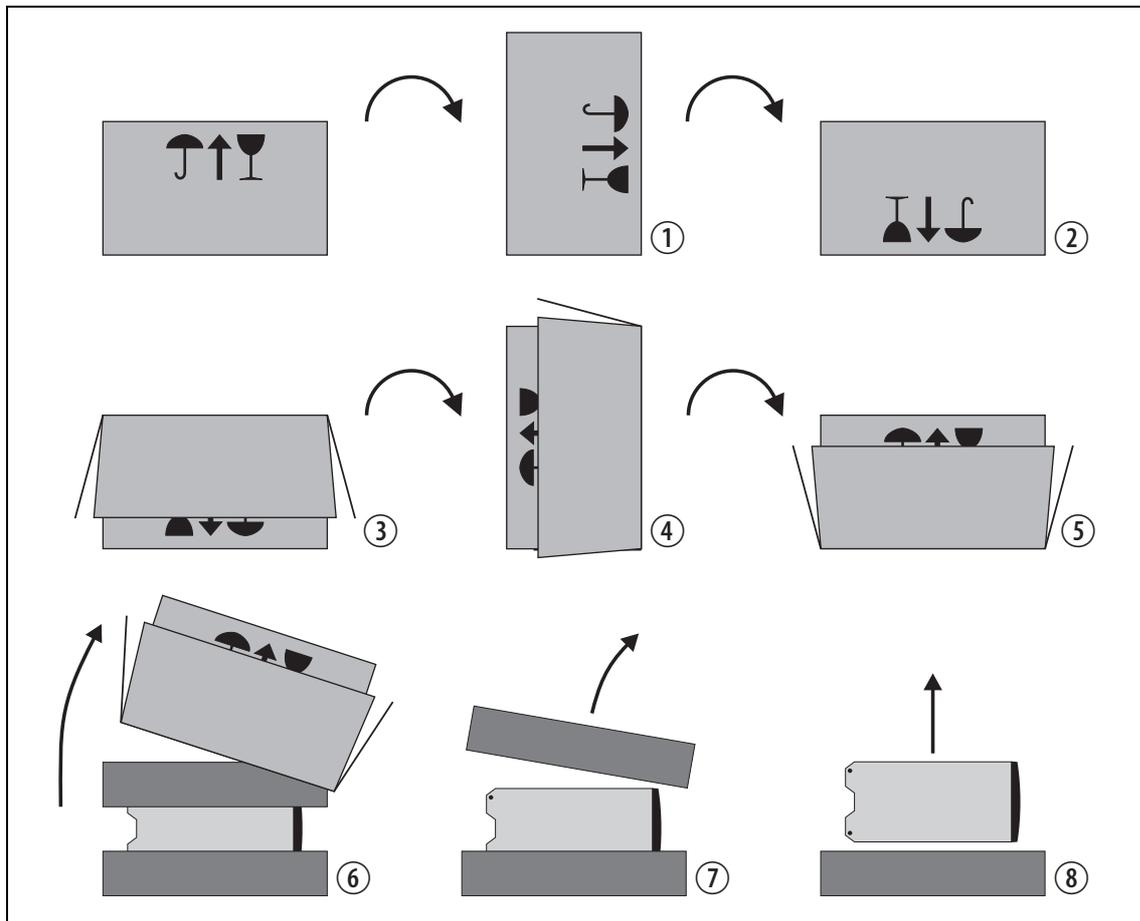
1. Rotate the carton carefully onto its side ① and then onto its top ②.
