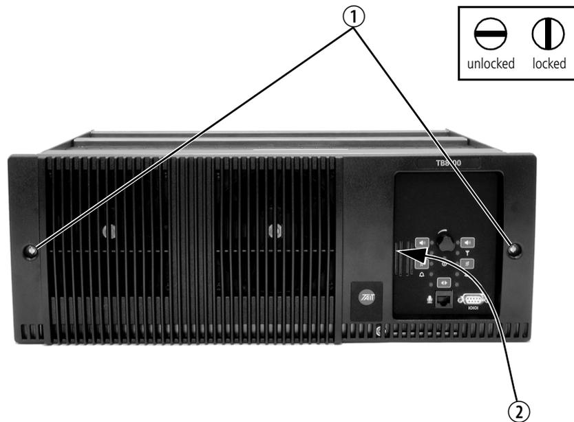
2. While supporting the left end of the front panel, place your fingers in the recess provided on the left side of the control panel opening ② and pull the right end of the front panel away from the subrack. You will need to overcome the resistance of the spring clip securing the front panel to the control panel.
