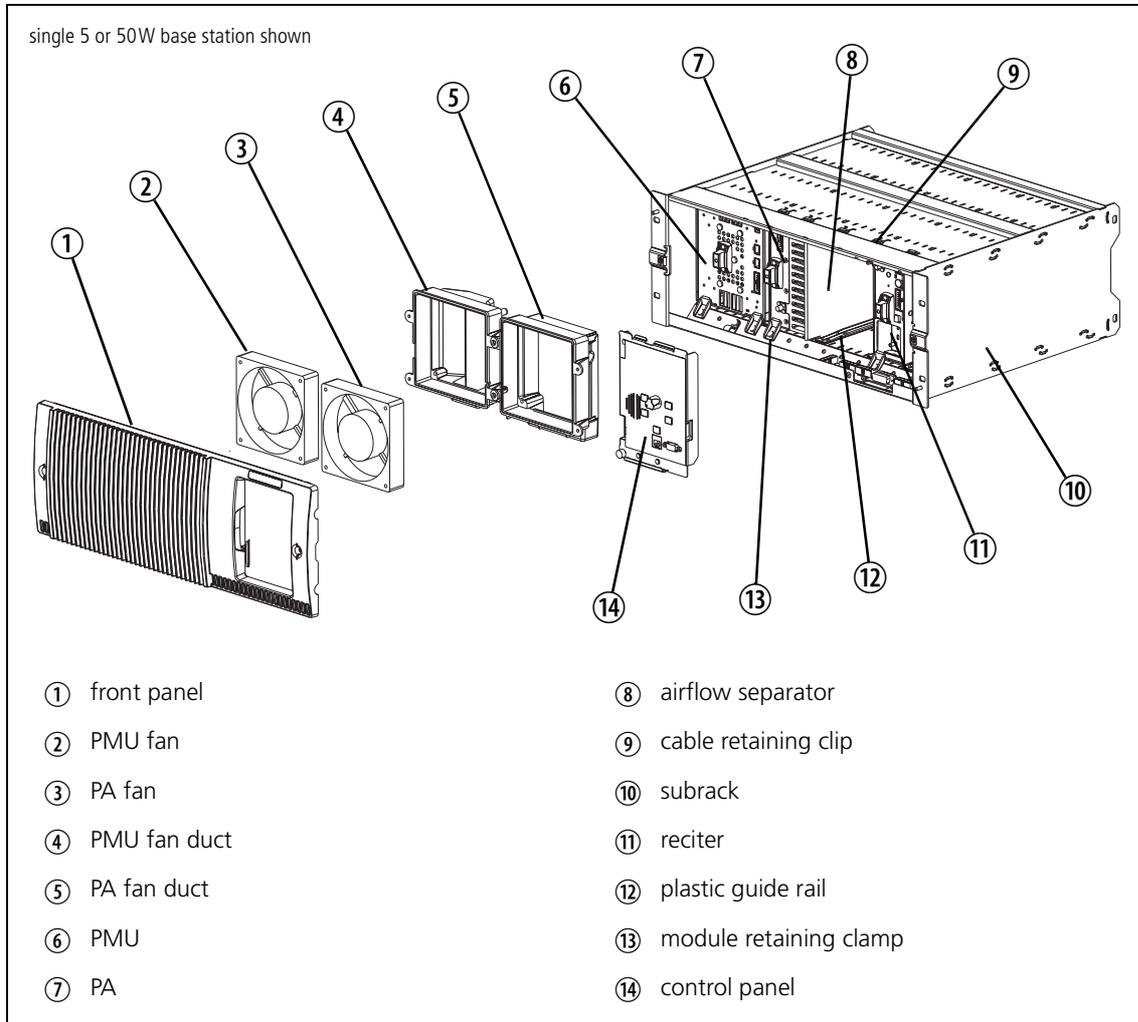
The front panel can be easily removed from the subrack by undoing two quick-release fasteners. Once the front panel is removed, the control panel can also be removed from the subrack by undoing a single screw. Refer to [“Replacing Modules” on page 43](#) for more details.
