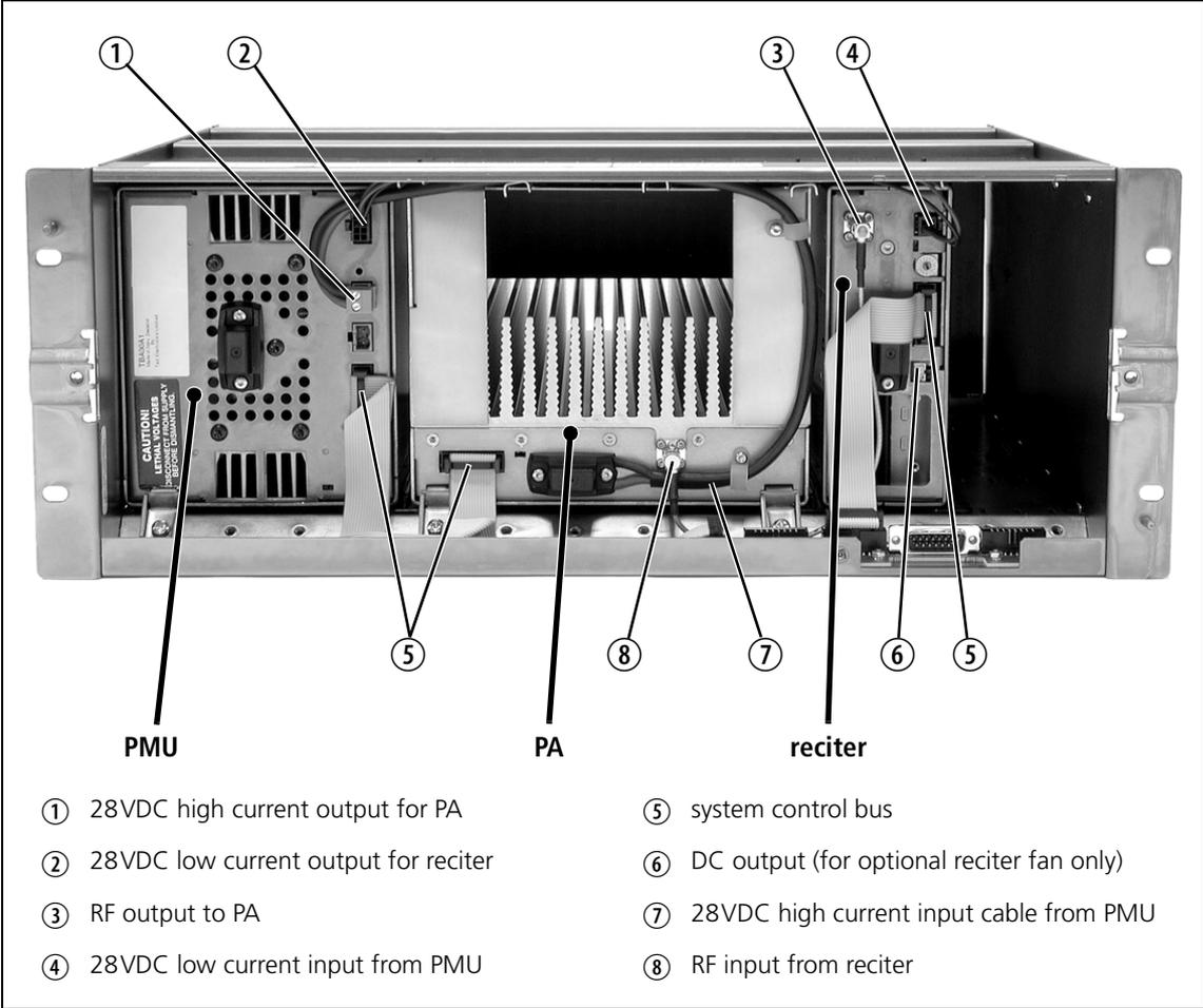
**Figure 6.3 Dual 5 or 50W Base Station Inputs and Outputs - Rear View**
