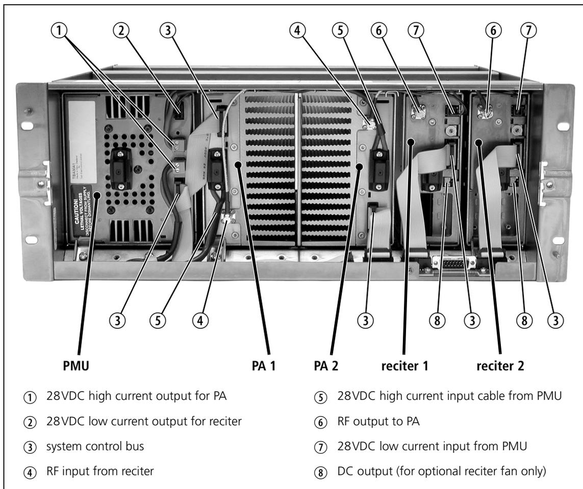
**Figure 6.2 Single 100W Base Station Inputs and Outputs - Front View**
