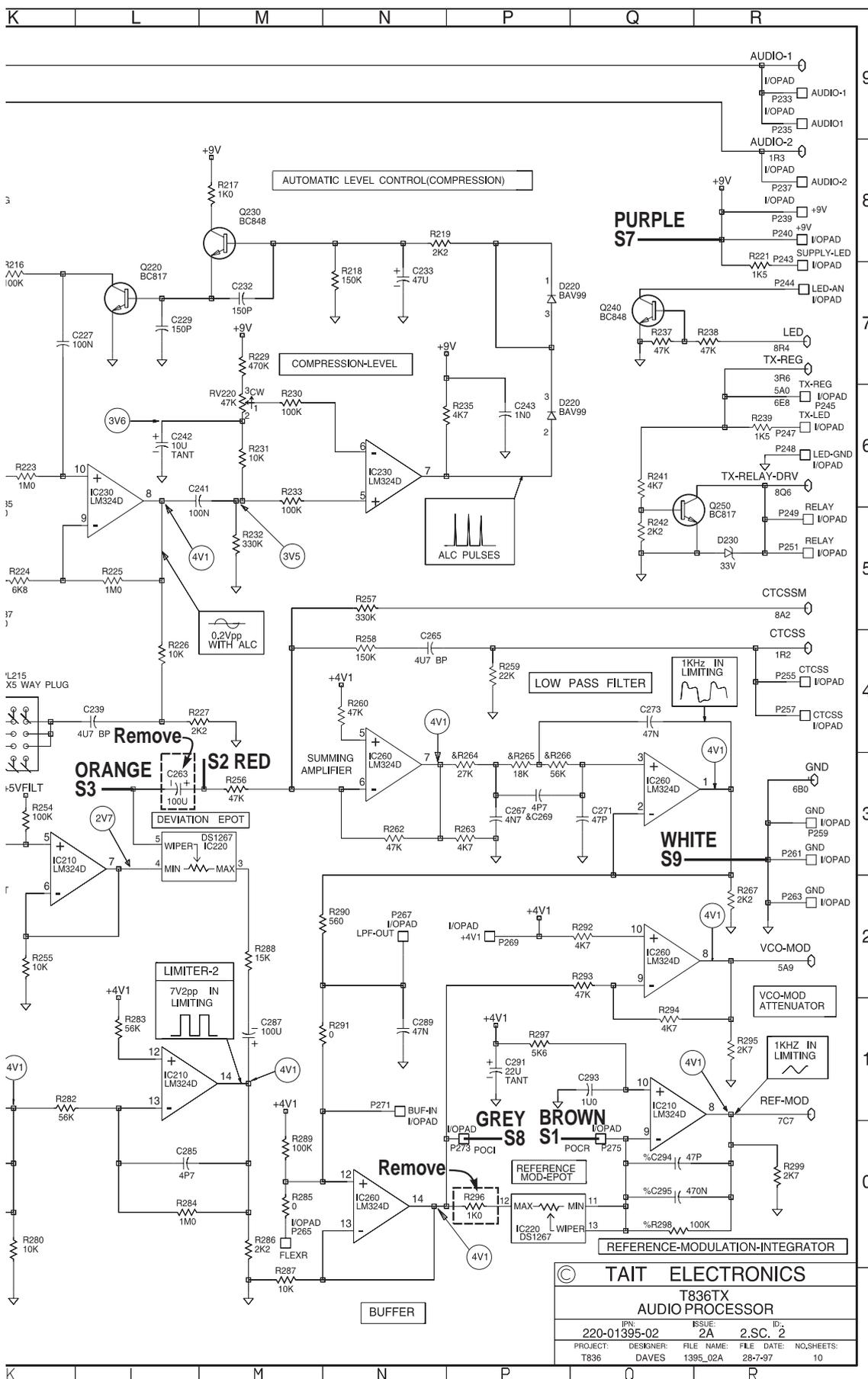
Figure 8 T800 Series II Transmitter Audio Processor Circuit Modifications
