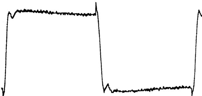
*Figure 7 100Hz VCO Control Line Waveform*
