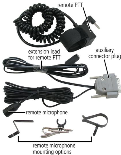
The TMAA10-04 hands-free kit plugs into the radio's auxiliary connector and can be used in conjunction with the radio's rugged microphone. When hands-free operation is required, the user activates the PTT using the conveniently located remote PTT key, and the remote electret microphone replaces communication through the usual rugged microphone.
