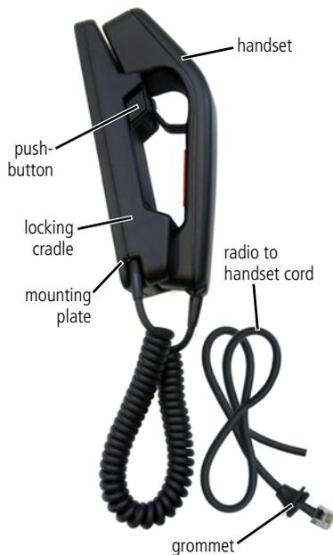
The TMAA10-02 handset provides the user with privacy and also improves the audio quality in noisy environments. The handset uses a dynamic microphone capsule, so the TMAA02-06 support kit for dynamic microphones must also be installed and configured for dynamic microphone operation.
