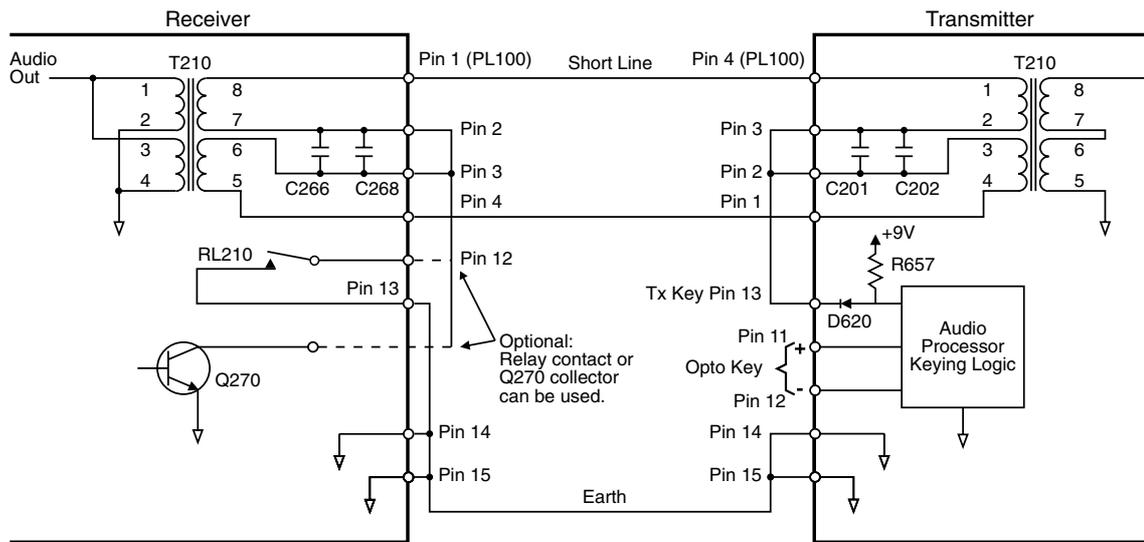
Figure 5.1 DC Loop Keying With Common Earth
