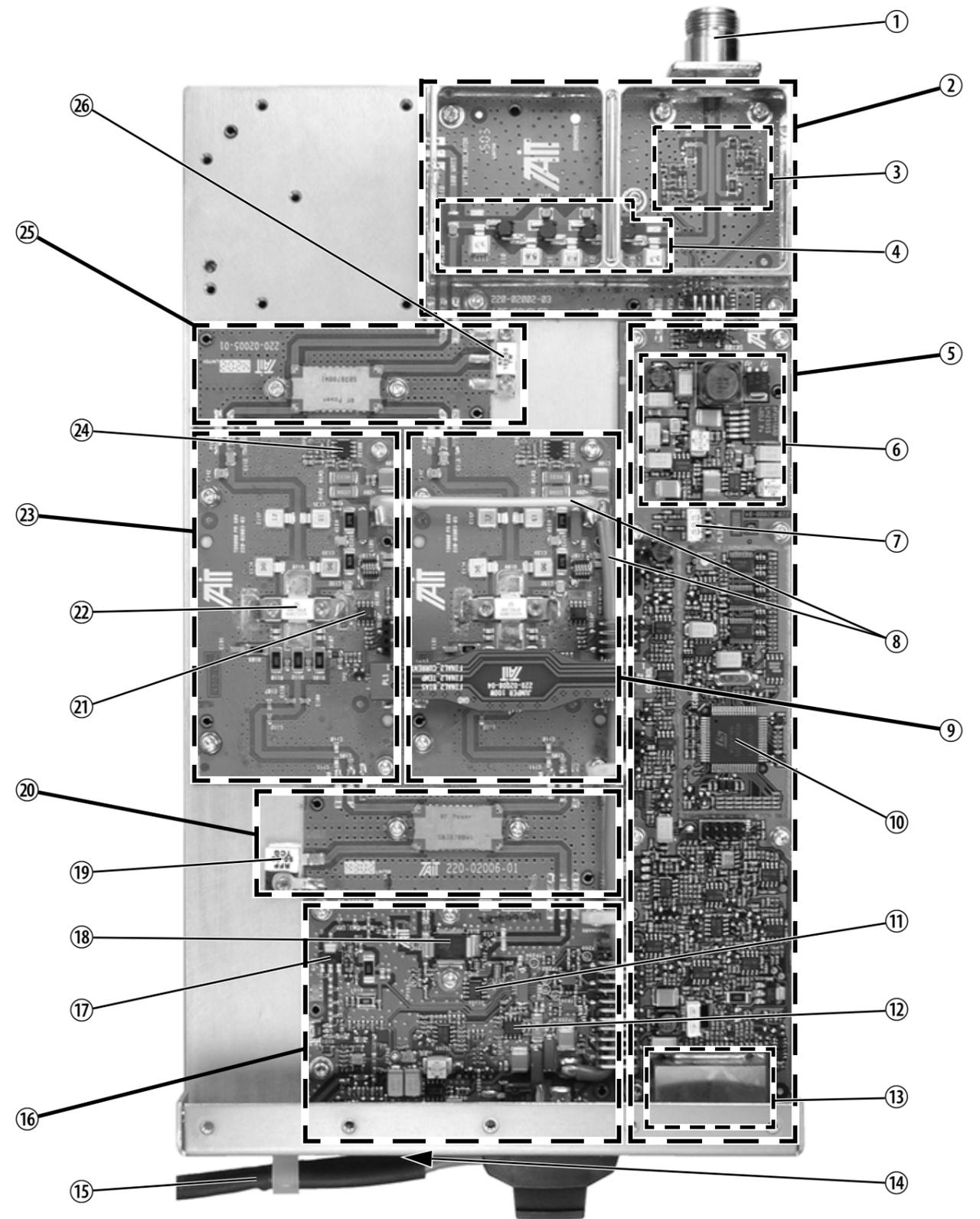
**Figure 7.4 Identifying the circuitry on the 12V PA boards**
