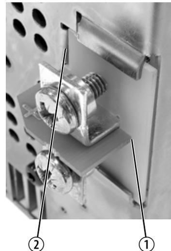
7. Refit and tighten the M4 Torx screw grounding the rear panel to the AC converter board.
