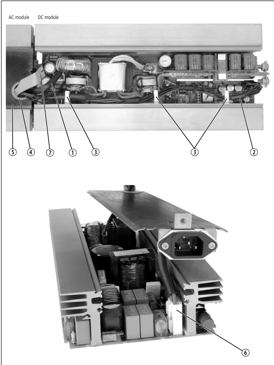
Figure 14.3 Reconnecting the AC and DC modules
