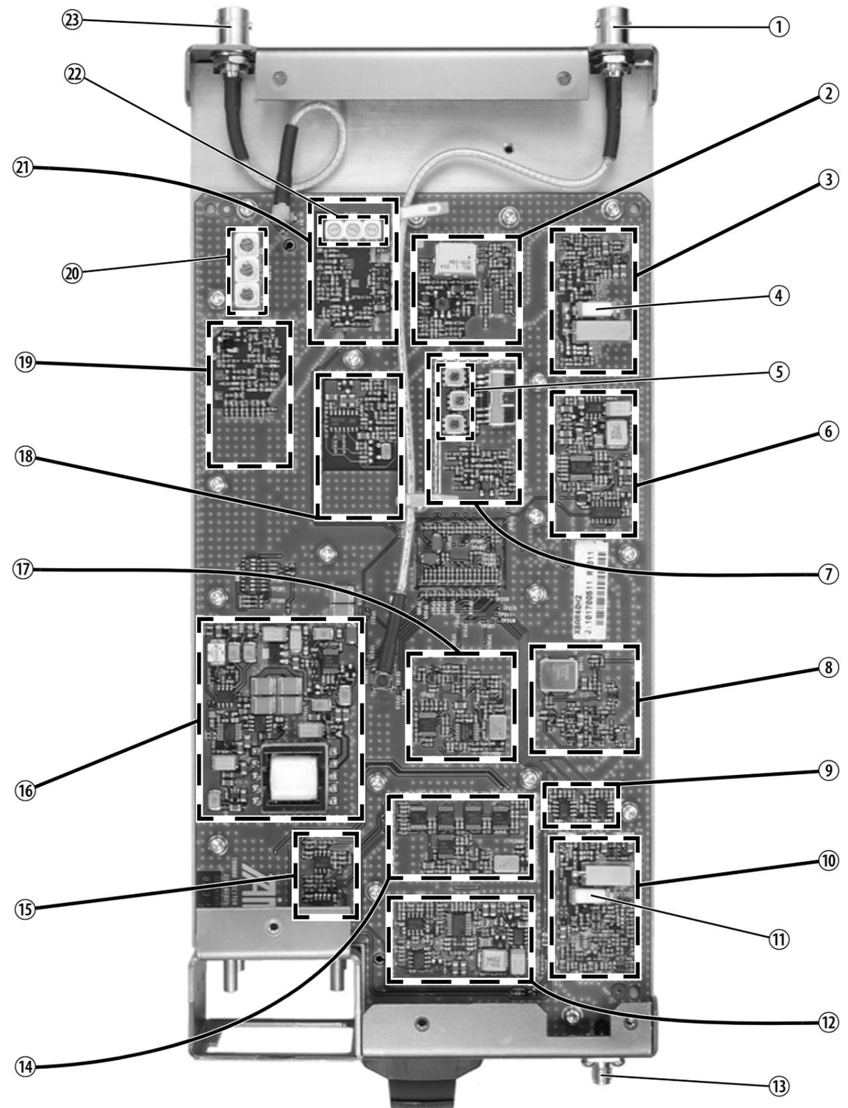
**Figure 2.17 Identifying the circuitry on the RF board - K and L bands**
