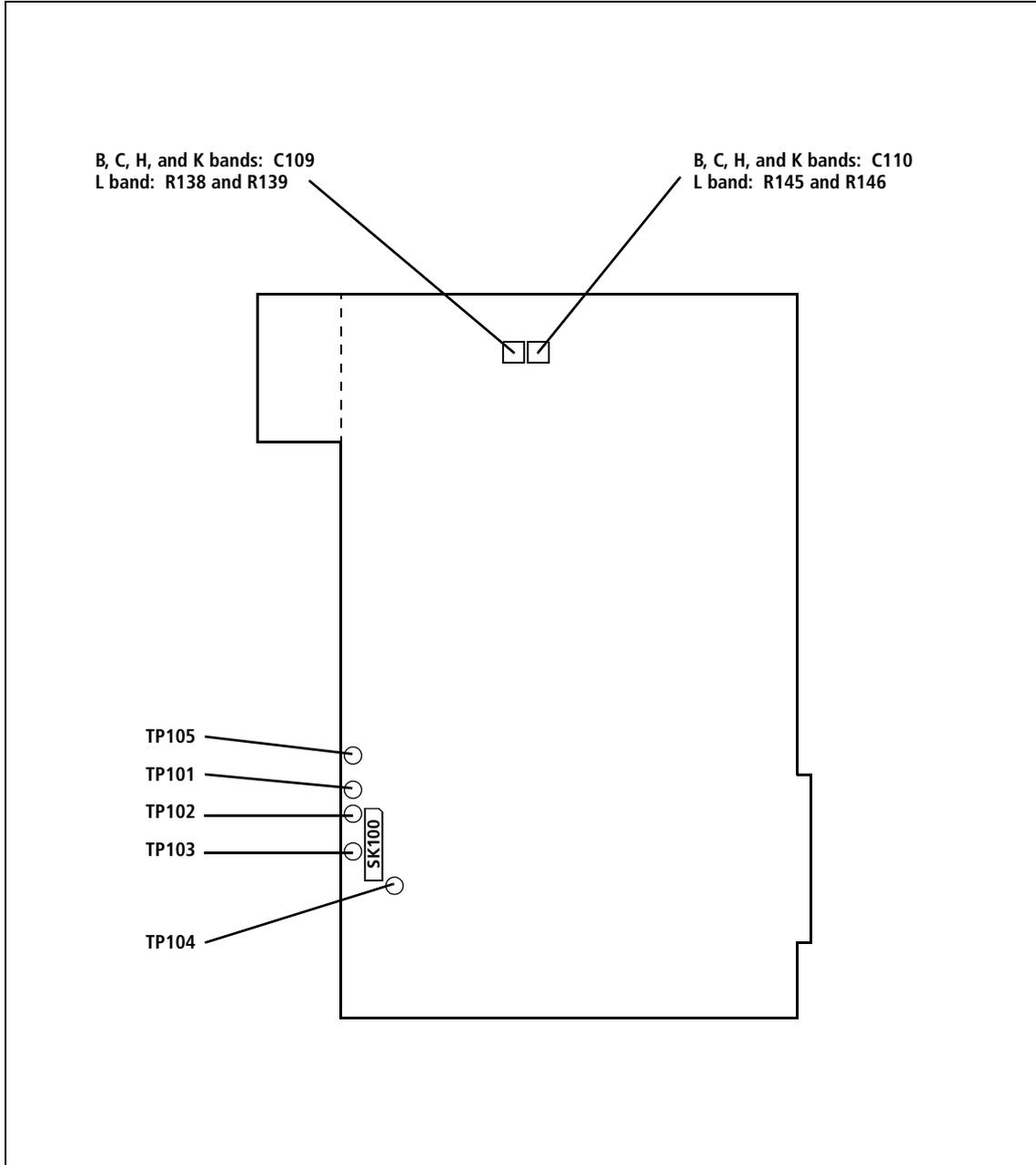
**Table 8.4 Placement of the input coupling components according to frequency band**
