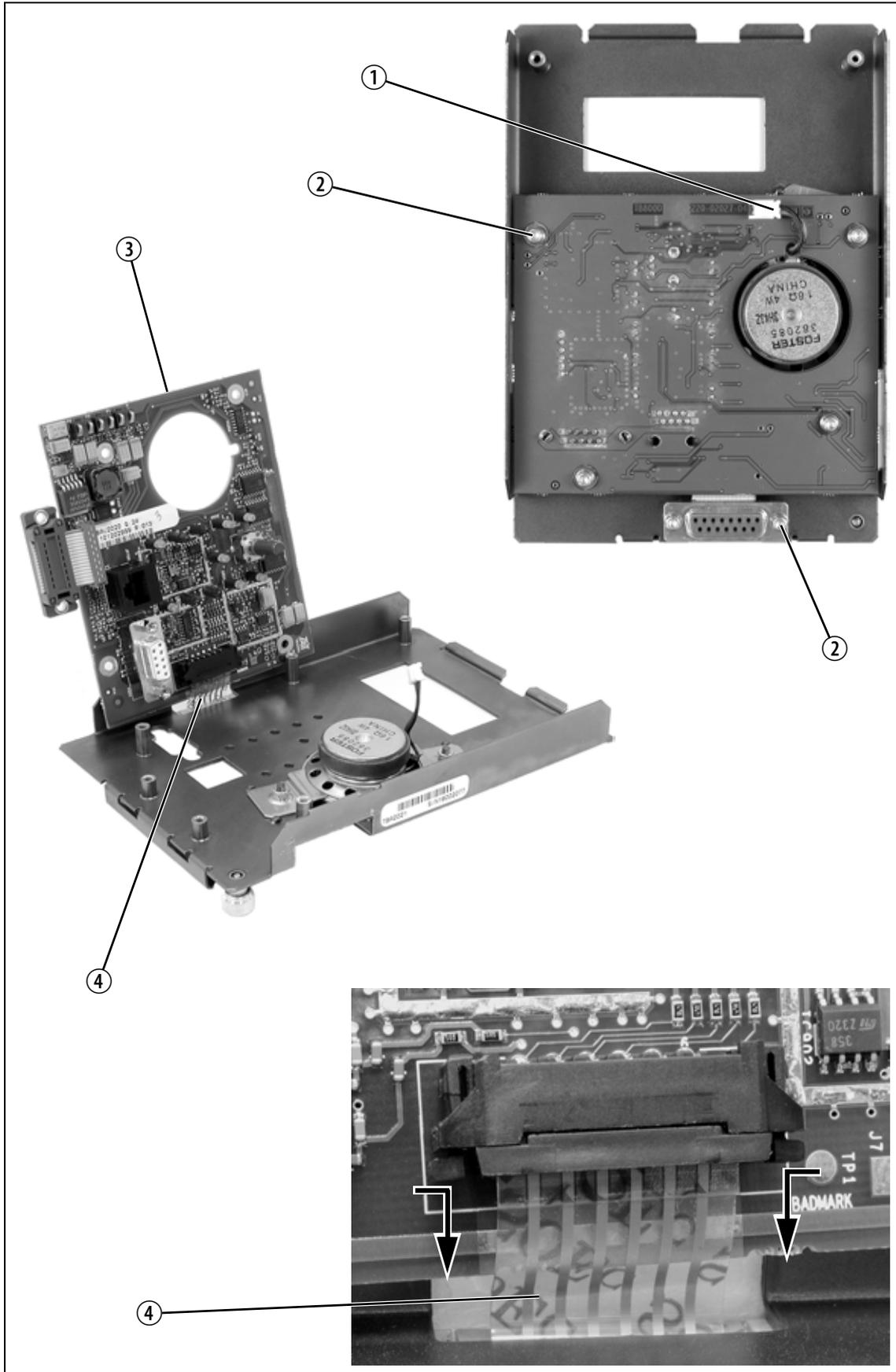
**Figure 18.2 Reconnecting the flexible connector**
