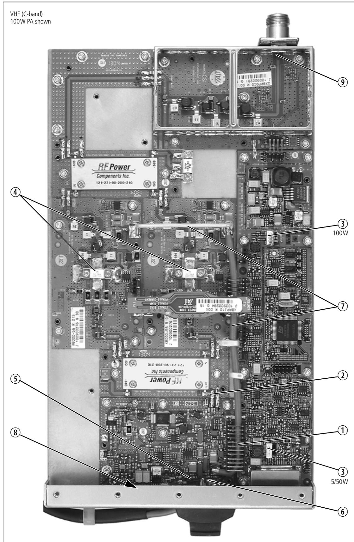
**Figure 8.7** Additional visual inspection points for a 12V PA
