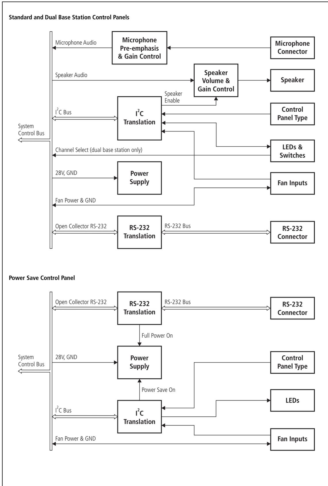
**Figure 17.2 Multi-reciter control panel high level block diagram**
