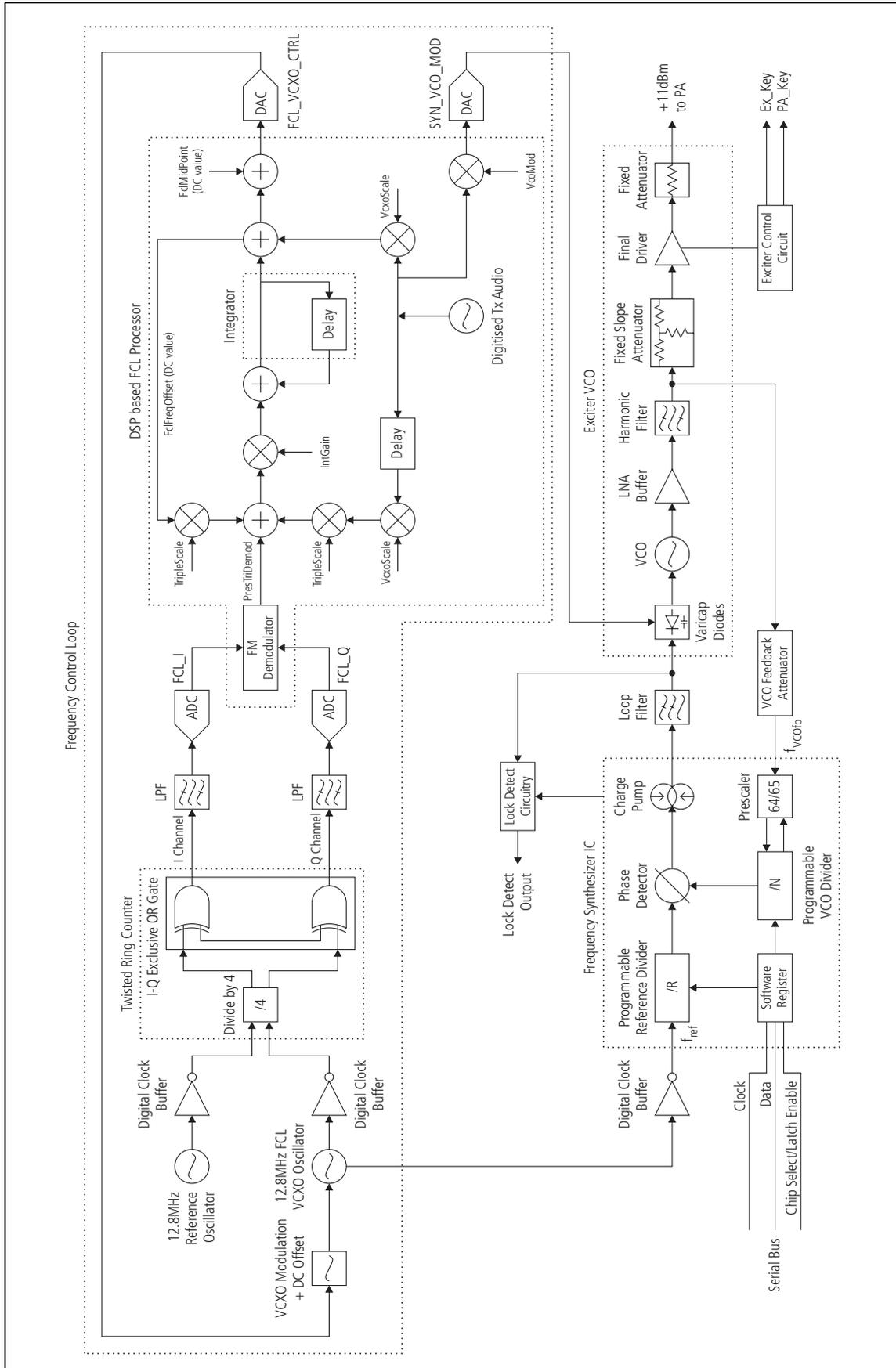
Figure 2.11 Reciter exciter synthesizer modulator block diagram - K and L bands
