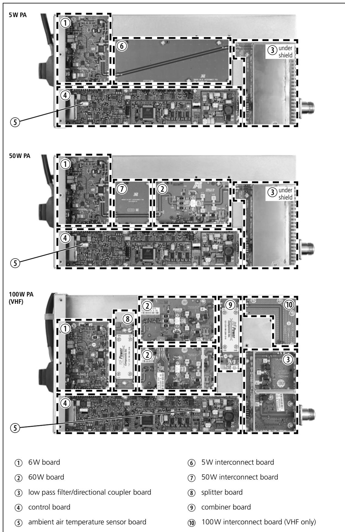
**Figure 8.2 Identifying the circuit boards in a 12V PA**
