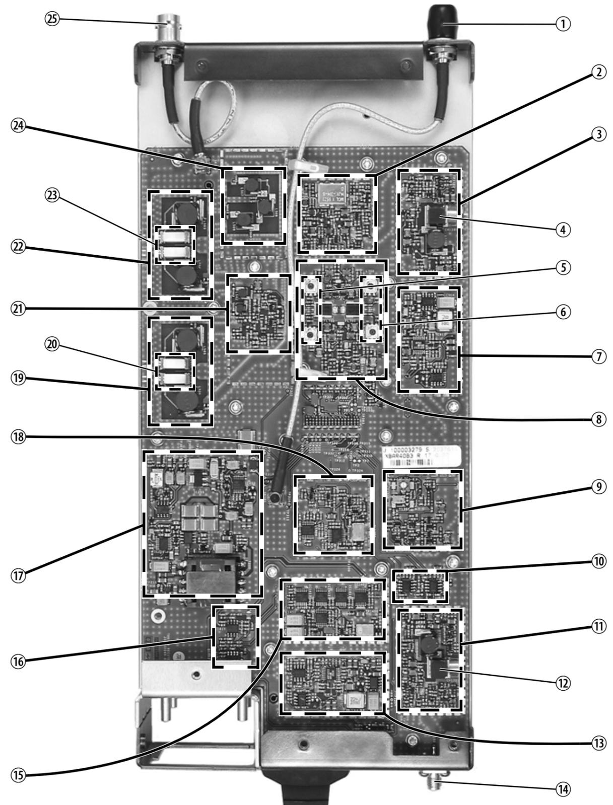
**Figure 2.16 Identifying the circuitry on the RF board - H band**
