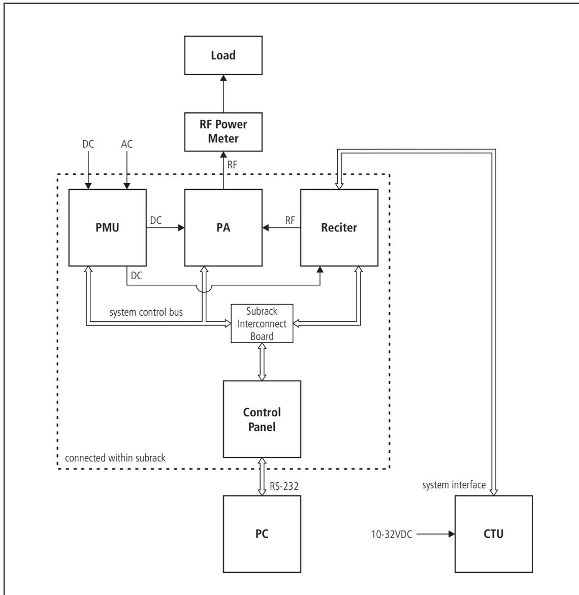
**Figure 8.4 Recommended test equipment set-up for initial checks - 12V PA**
