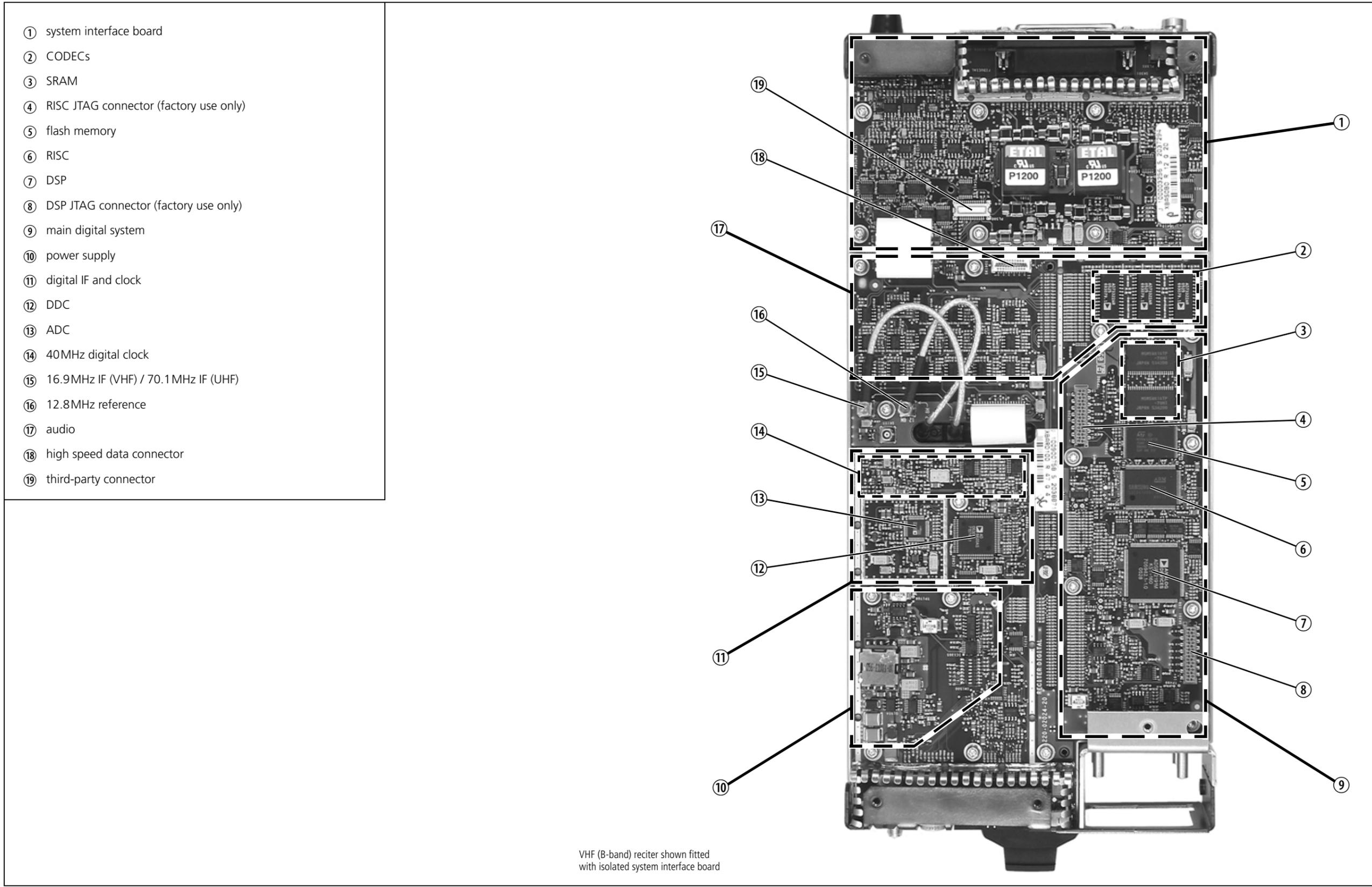
**Figure 2.15 Identifying the circuitry on the RF board - B and C bands**
