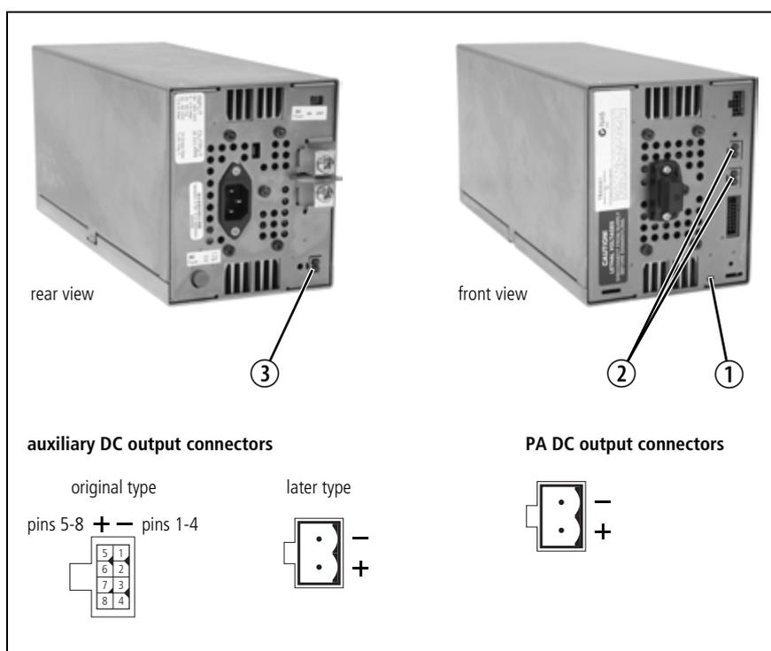
5. Check the output voltage at either PA connector ② on the front panel. If the PMU is fitted with an auxiliary power supply board, also check the output voltage at the connector ③ on the rear panel. The voltages should be as listed in [Table 13.1](#).
