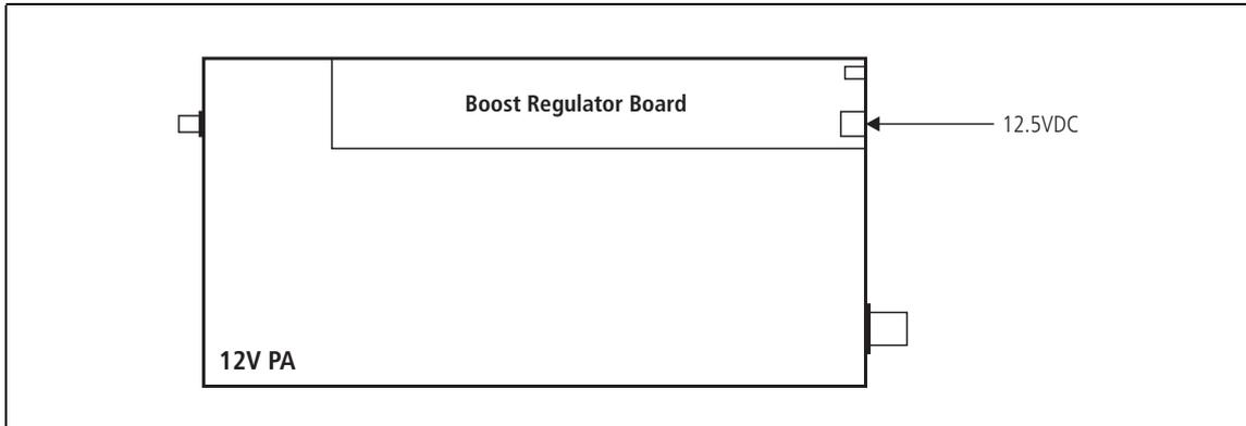
**Figure 8.16 Location of test points on the boost regulator board**
