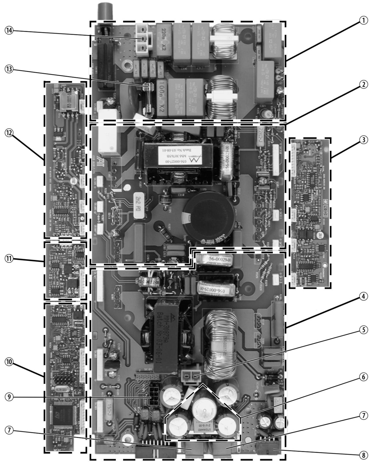
Figure 12.6 Identifying the circuitry in the DC module
