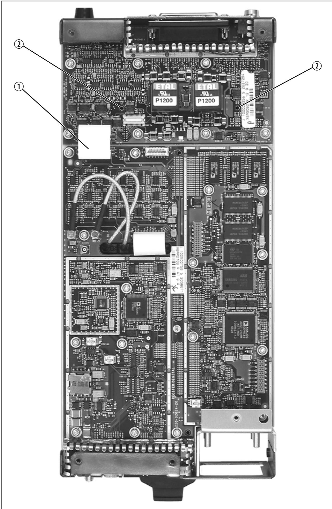
**Figure 5.2 Reconnecting the flexible connector**
