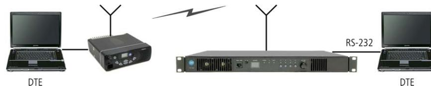
Using a TB7100 base in this configuration has the advantages of a higher duty cycle, higher transmit power and the possibility of duplex transmission, (although the TM8000 is semi-duplex so two would be required).
