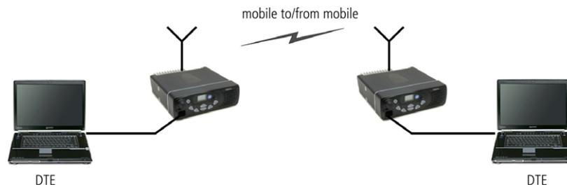
In this configuration the DTE is connected to the TM8000 via the serial port, data is sent from DTE to DTE via the TM8000 radio modems.
