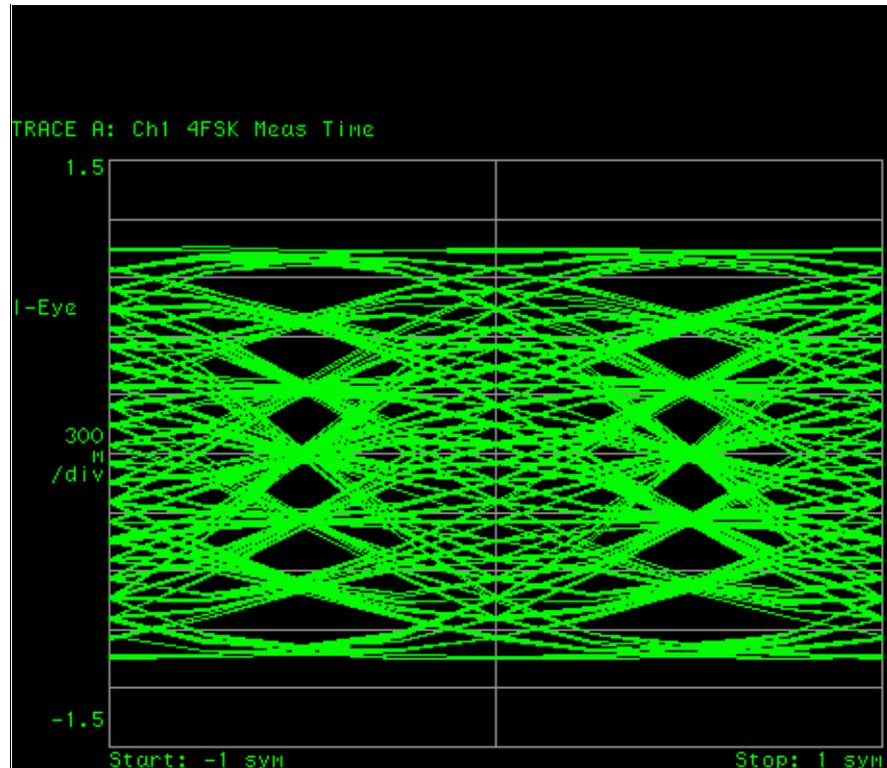
Like C4FM, this is a four-level FSK scheme, but can achieve higher data rates while maintaining compliance with ETS300-113 ACP. This scheme is a form of minimum shift keying, and hence is a subset of MSK.
