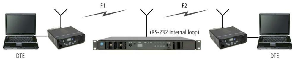
In this configuration, data is sent from the DTE to TM8000 to the TB7100. The data is then decoded by the TB7100 receive module and sent to the serial port where it is “looped” back to the transmitter module.
