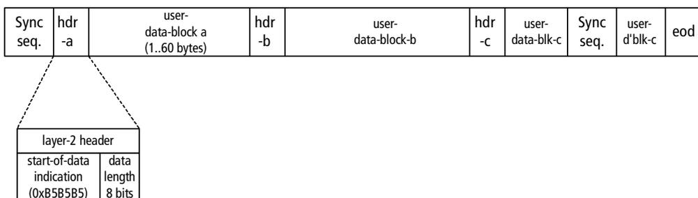
The eod (End Of Data) indication merely provides a lead-out delay to ensure that the data is completely sent before the transmitter is turned off.
