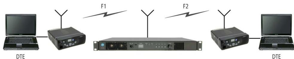
In this configuration, the TB7100 acts as a talk through repeater. When the receive gate of the receive module opens, the transmit module starts transmitting and audio is passed from the receive module to the transmit module. This configuration is:
