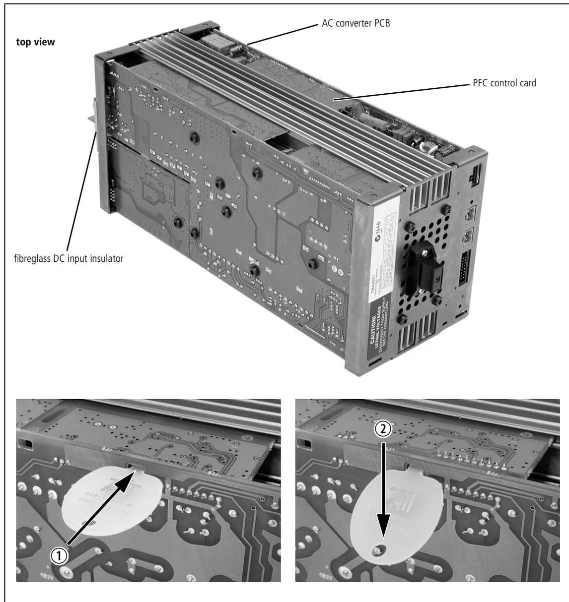
3. Remove Q304 and R336 from the AC converter PCB, as shown in [Figure 2](#).
