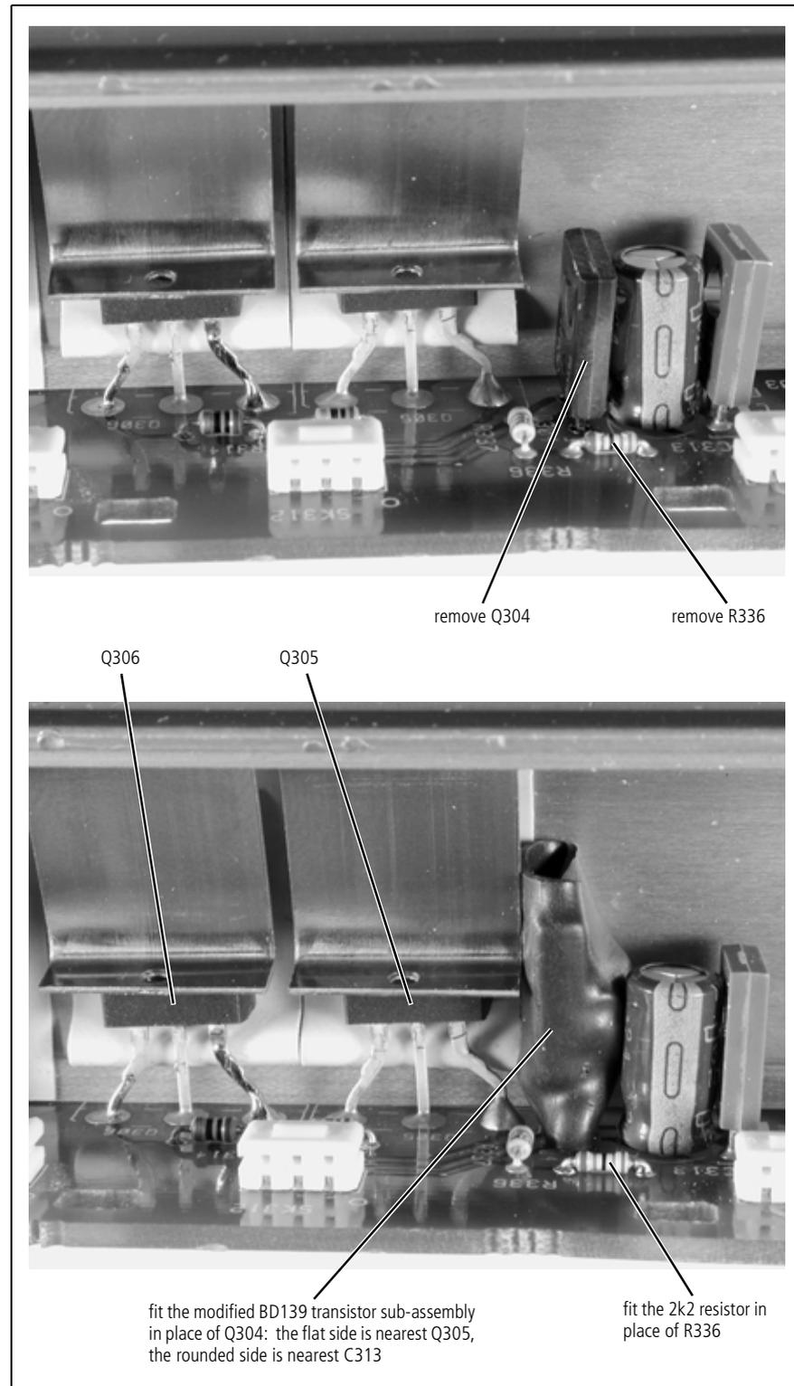
5. Fit the 2k2 resistor in place of R336, as shown in [Figure 2](#).
