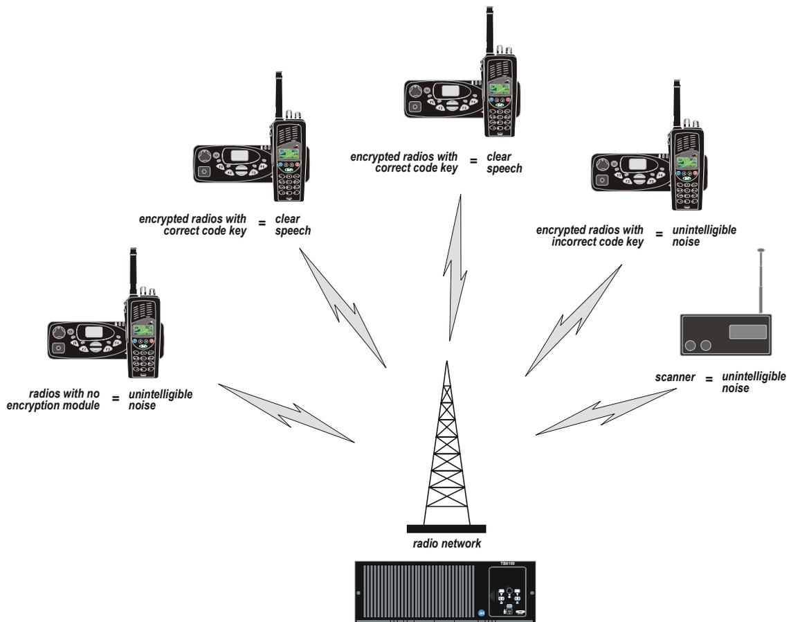
Whether or not a radio transmission is encrypted is the user's choice. When the encryption mode is selected, the radio sends and receives encrypted calls to and from other radios with compatible encryption module and settings. However, even when encryption is not selected, an encryption-enabled radio will always decode encrypted communication from any radio with compatible modules and settings.
