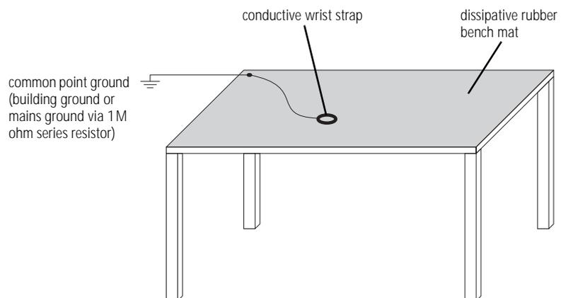
You can obtain further information on antistatic precautions and the dangers of electrostatic discharge (ESD) from standards such as ANSI/ESD S20.20-1999 or BS EN 100015-4 1994.
