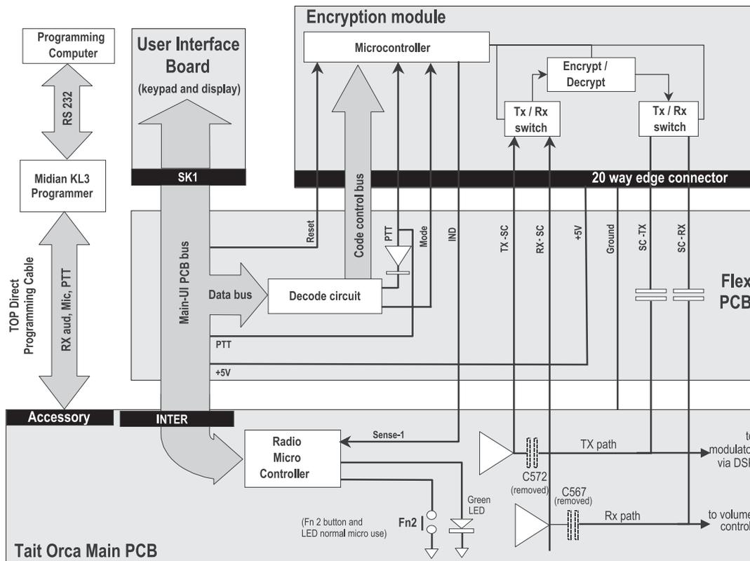
An addressable latch on the radio User Interface board is replicated on the encryption flex and driven by the same serial data bus. The radio micro uses four outputs of this latch to control the encryption code select bus. Two other outputs provide the PTT and Mode drives to the module. The remaining two pins function as normal for the User Interface board and are unused on the flex.
