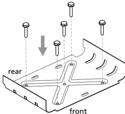
1. Use the drilled half of the metal cradle cover as a template to mark the holes for drilling.
