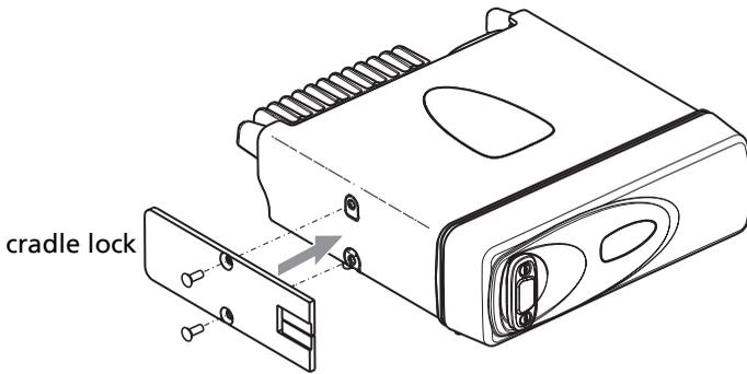
6. Attach the Cradle Lock to the side of the radio using the countersunk Torx M4×10 screws supplied, ensuring the recessed section is to the front, and facing out.
