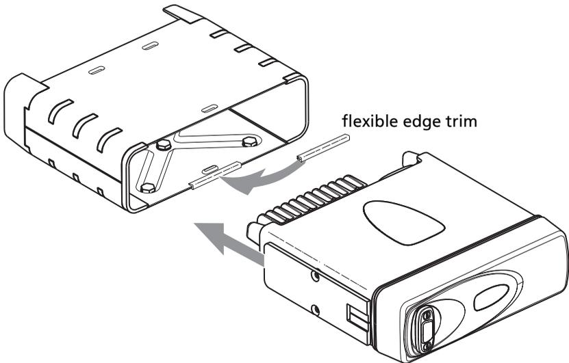
7. Slide the flexible edge trim onto the lower front edge of the cradle.
