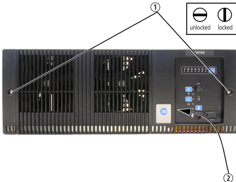
2. While supporting the left end of the front panel, place your fingers in the recess provided on the left side of the control panel opening ② and pull the right end of the front panel away from the subrack. You will need to overcome the resistance of the spring clip securing the front panel to the control panel.
