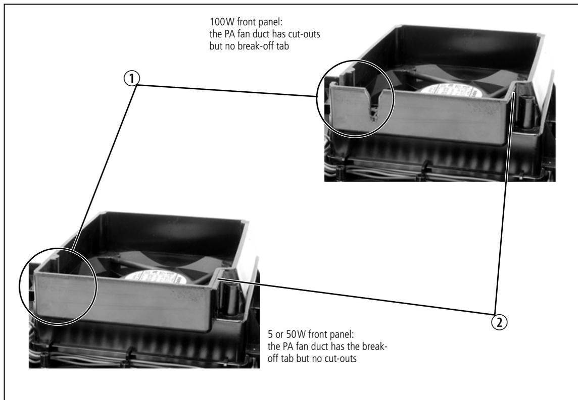
1. Before fitting the front panel, ensure that all cables are secured and positioned correctly so they are clear of the fan ducts (refer to [Figure 3.8 on page 52](#) and [“Appendix B – Inter-Module Connections” on page 123](#)). Otherwise the panel may not fit properly, or you may damage the cables.
