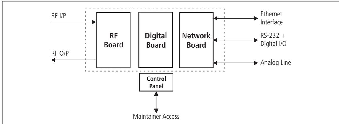
The RF board contains the receiver and exciter circuitry.
