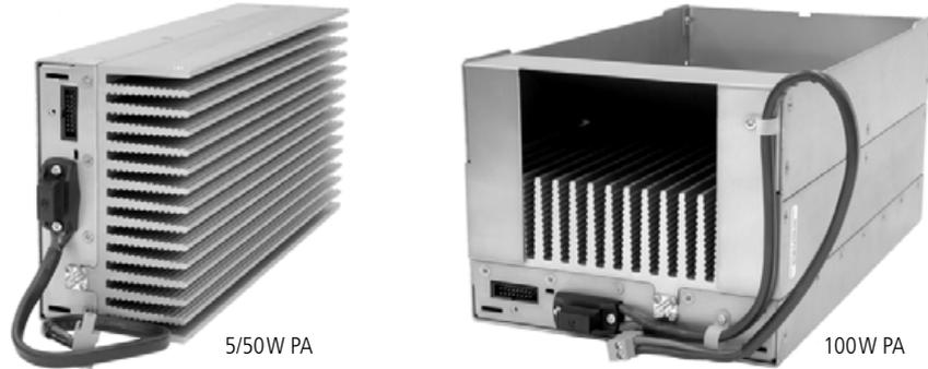
All three models are designed to operate on the 28 VDC output provided by the TB9100 power management unit. In addition, variants of the 5 W and 50 W models are available for DC-only operation. These two 12 V PAs are fitted with an internal boost regulator board, which converts the 12 V nominal DC input to a 28 VDC output to power the PA circuit boards. The boost regulator board also provides a 12 VDC output to power the reciter.
