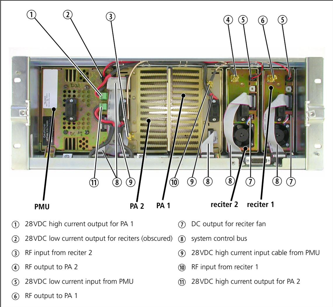
Special care should be taken when connecting the power cable from the PMU to PA 2. The cable should be shaped in such a way that it does not come into contact with the subrack interconnect board. Refer to the diagram below for more detail.
