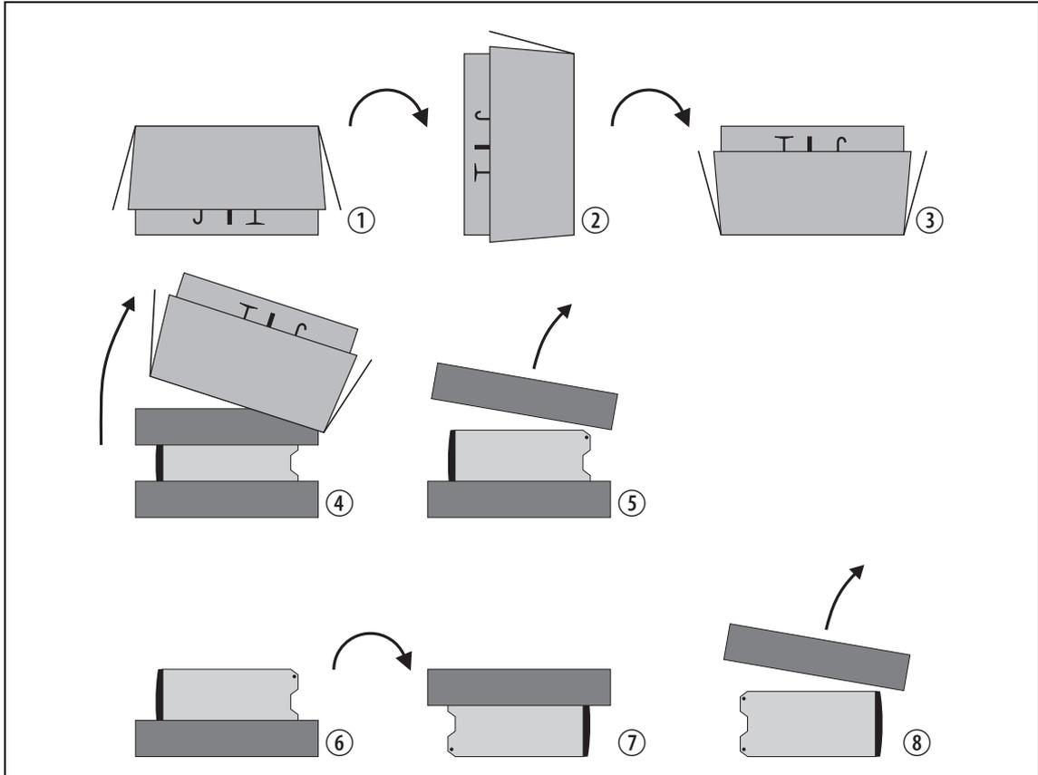
1. Cut the tape securing the flaps at the top of the carton and fold them flat against the sides ①.
