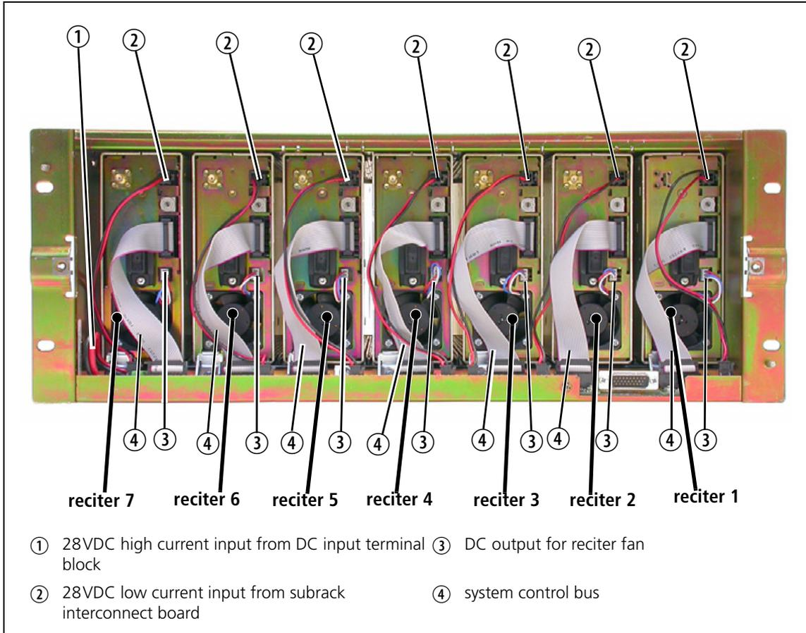
The following diagram shows the subrack interconnect board connections for this configuration.
