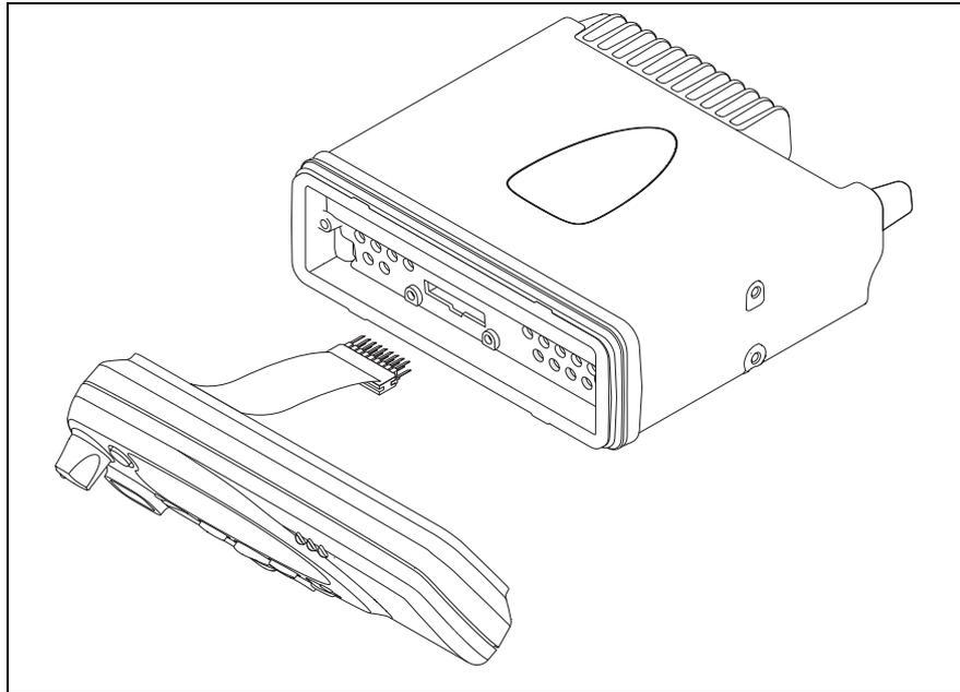
1. Plug the control-head loom onto the control-head connector.
