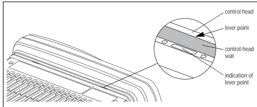
On the underside of the radio, two lever points are indicated on the radio body by a dot-dash-dot pattern (○ — ○). The lever point is between the control-head seal and the control head.
