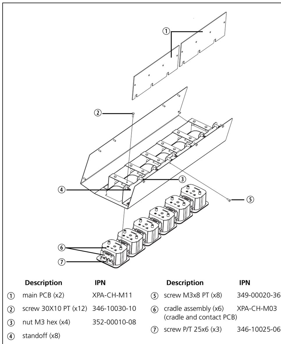
Figure 15.5 Parts of the multi-charger base assembly
