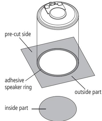
**Figure 5.10 Fitting the speaker**
