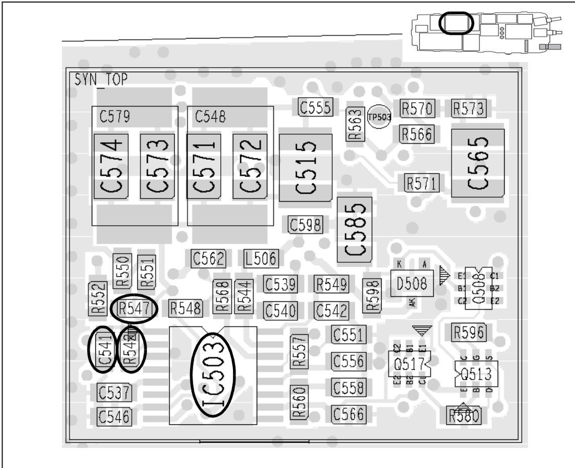
Figure 9.16 Synthesizer components under the PA EX TOP can (VHF radio, top side)
