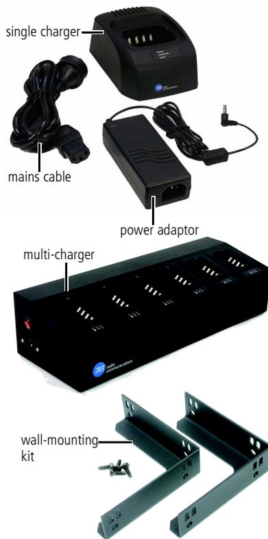
There are two battery chargers available for the TP9100: the TPA-CH-001 desktop charger for charging single batteries, and the TPA-CH-011 multi-charger for charging any combination of up to six batteries. The following Tait batteries can be charged:
