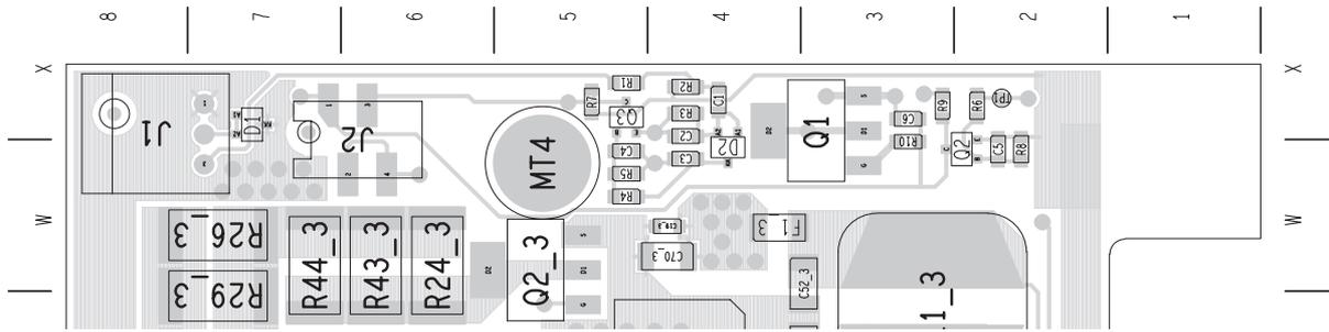
Figure 15.8 Components of the middle charger slot
