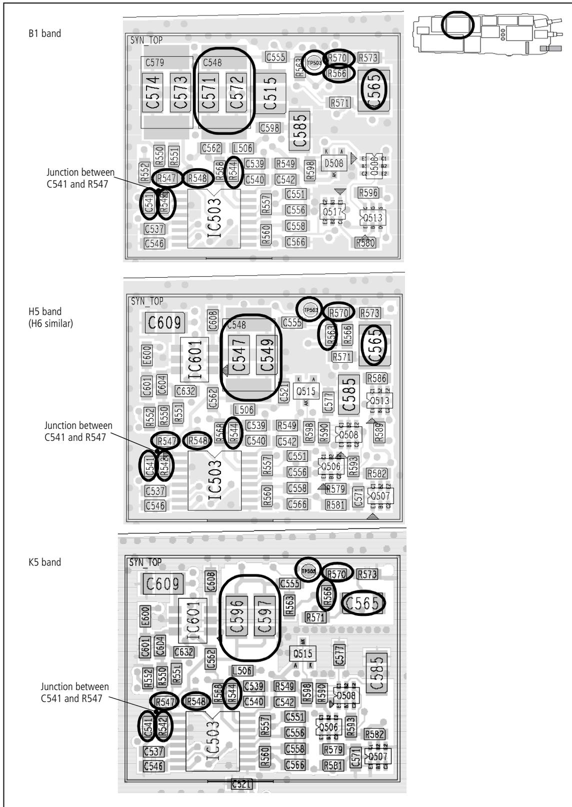
Figure 9.9 Synthesizer components under the SYN BOT can (bottom side)
