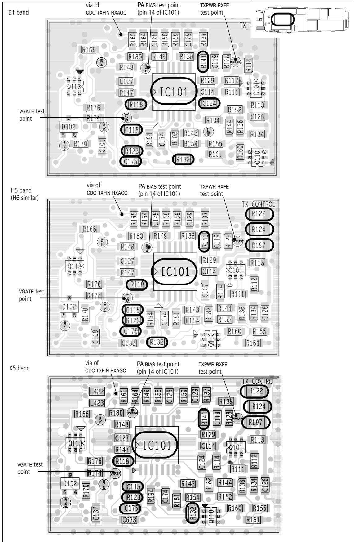
If the voltage measured in Task 10 is correct but not the current, either the PA or the shaper and level shifter for the PA is suspect.
