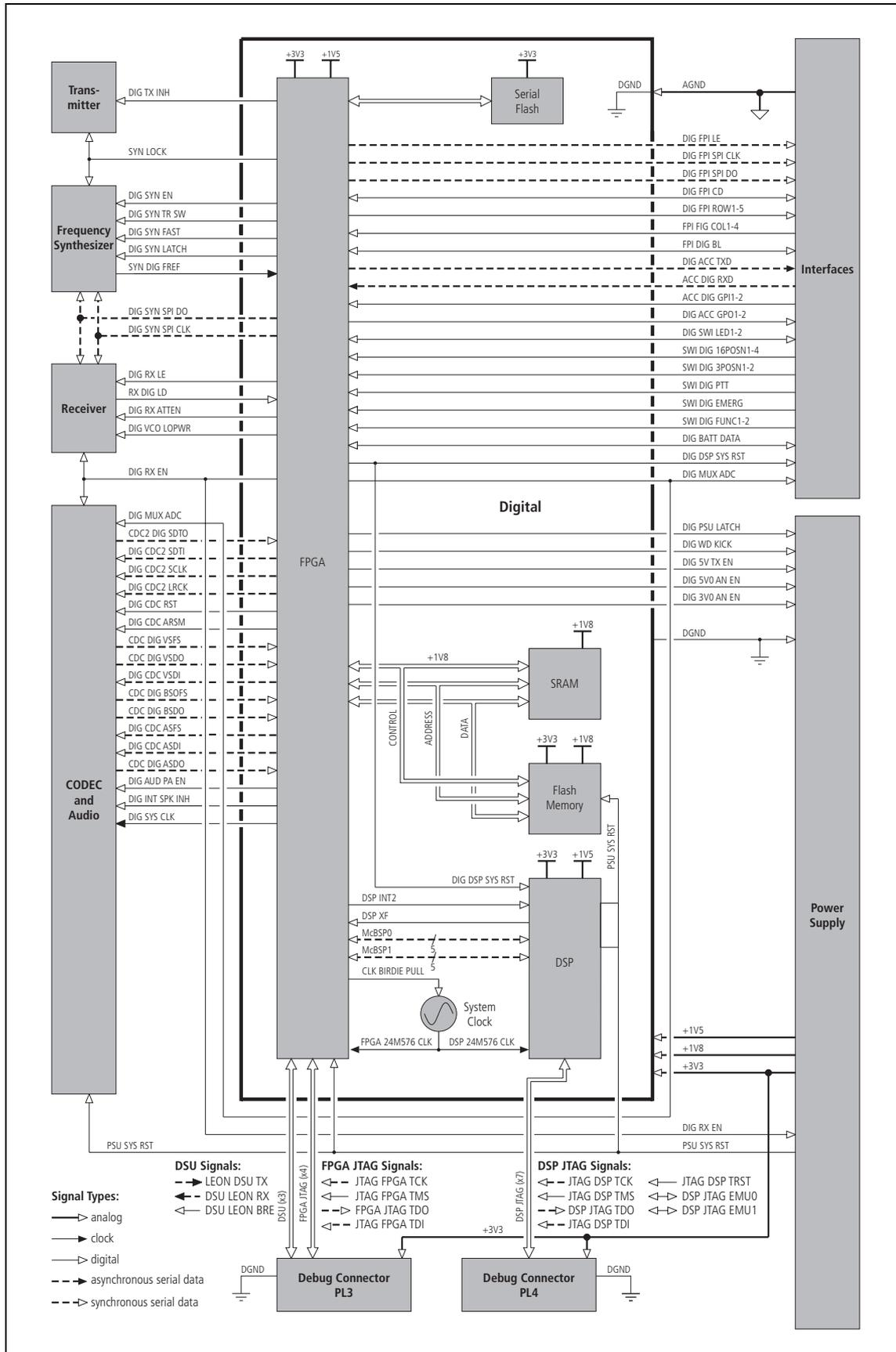
Figure 3.10 Block diagram of the front-panel interface board circuitry
