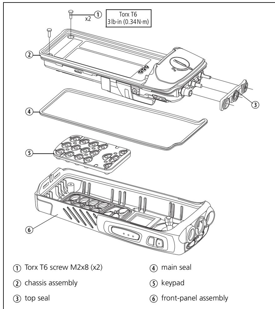
2. Place the top seal ③ over the power/volume potentiometer, 16-way/3-way selector switch, and antenna SMA connector.
