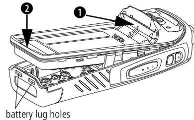
5. Look through the holes in the top of the front-panel assembly and check whether the top seal ③ is placed correctly around the power/volume potentiometer, 16-way/3-way selector switch, and antenna SMA connector
