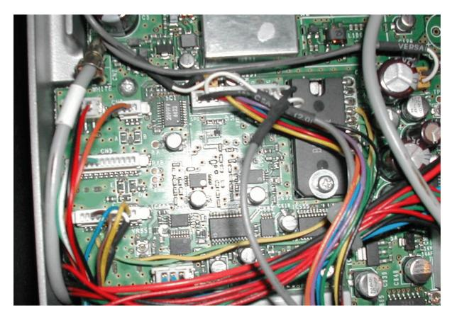
10) Plug the small 9 way connector of the GPS/RS232 cable into the 9 way connector on the SC90 board Making sure the wires will not be trapped by the cover when it is replaced.
