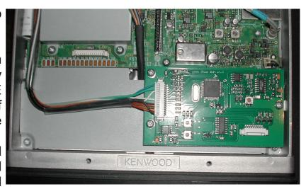
will be relatively hard to screw in the first time as they cut the thread in the chassis mounts. When re-inserting the screws after they have been removed be very careful to ensure they use the existing cut thread.
