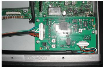
Run this cable down the left hand side of the radio to exit through the rear panel of the TK-90 (remove the exit hole sticky cover - item 23 - see Exploded View in the TK-90 Technical Manual). Ensure the cable tie on this cable is on the inside of the rear panel for strain relief purposes.
