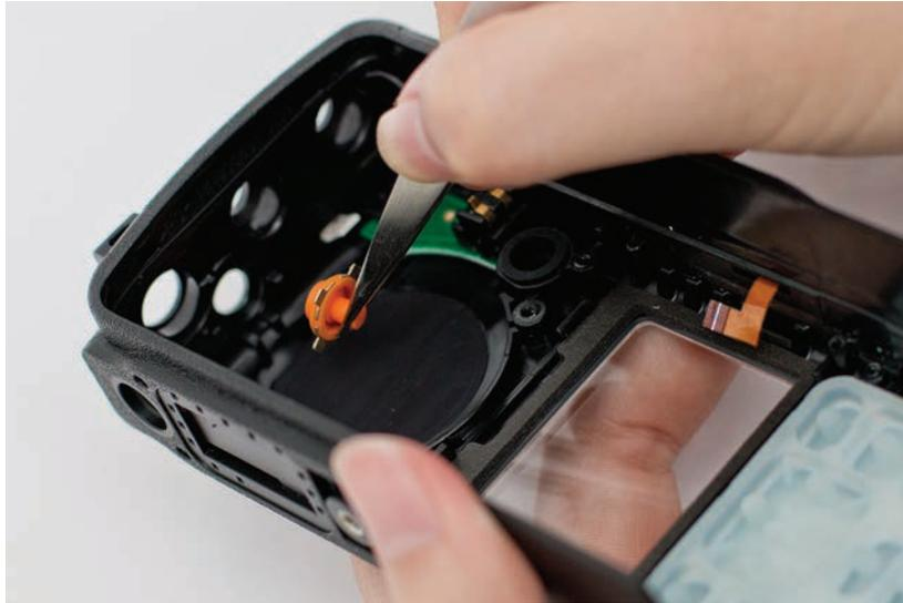
*Figure 5-24. Emergency button removal*
