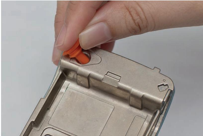
*Figure 5-13. RF rubber plug removal*
