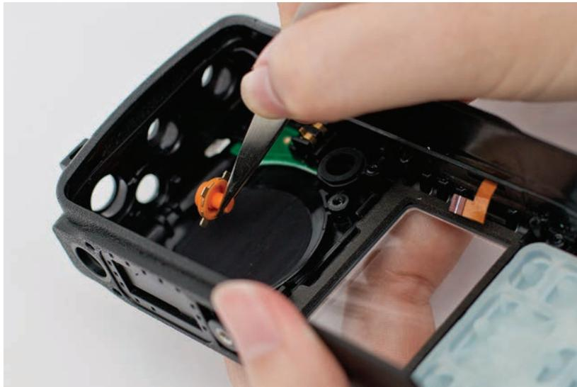
*Figure 5-27. Emergency button reassembly*
