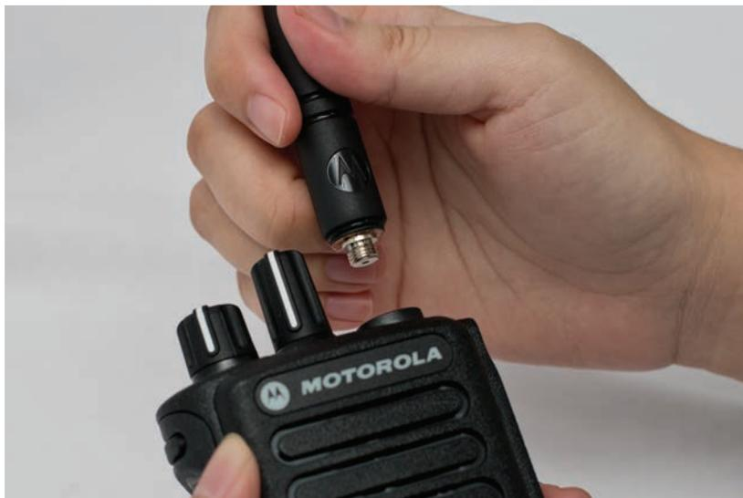
Figure 5-2. Antenna removal.
