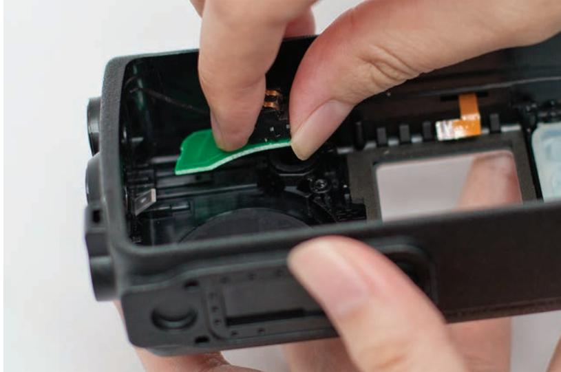
*Figure 5-26. Bluetooth GPS antenna reassembly*
