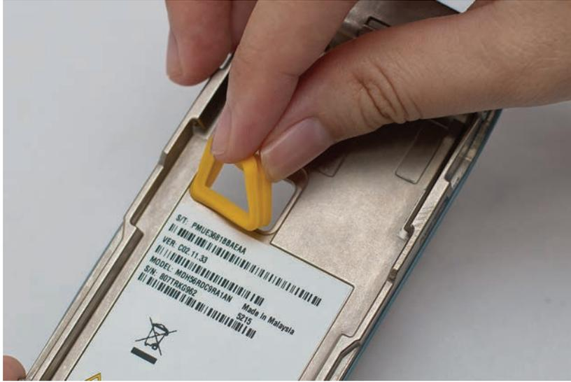
*Figure 5-12. Battery contact seal removal*
