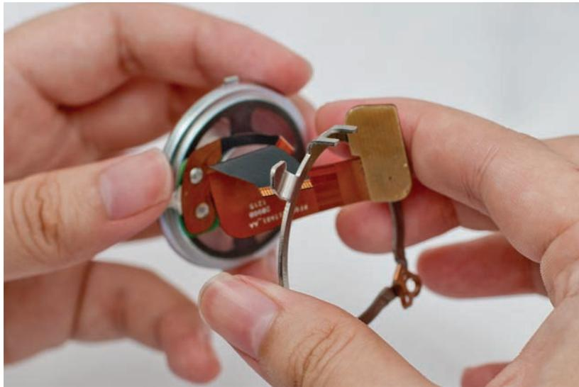
Figure 5-28. Speaker retainer reassembly
