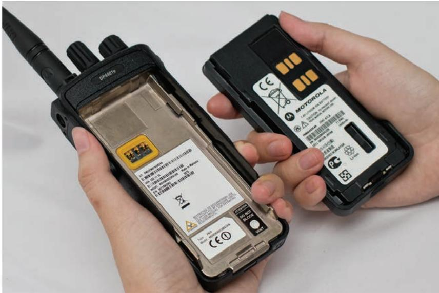
Figure 5-1. Battery removal
