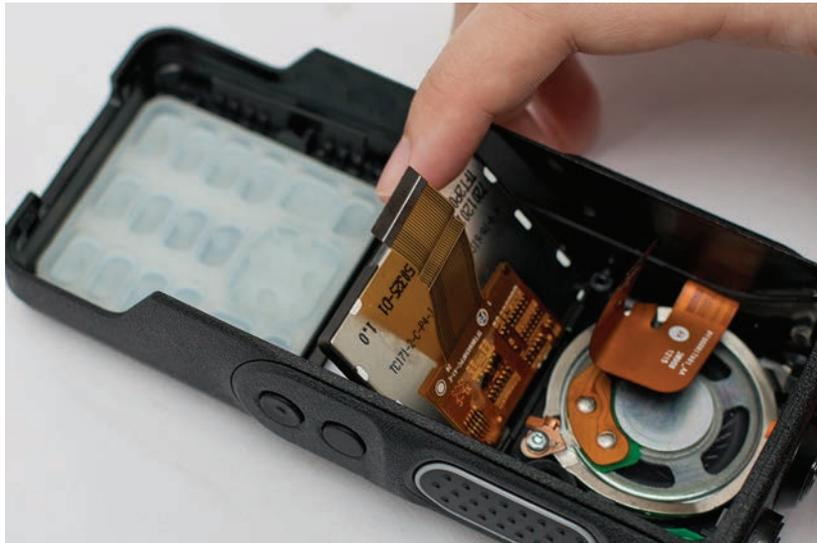
*Figure 5-19. Display module removal*
