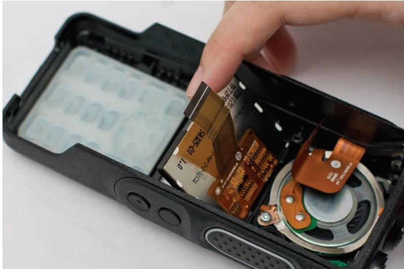
Figure 5-31. Display module reassembly
