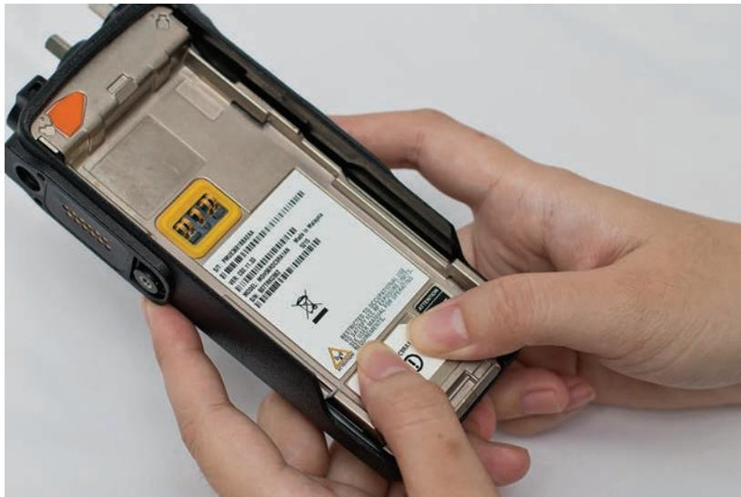
Figure 5-39. Chassis reassembly
