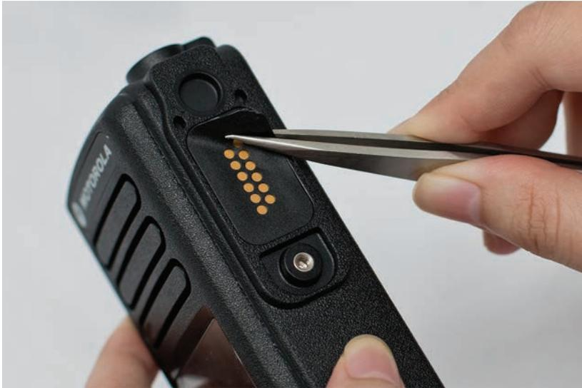
*Figure 5-20. UC escutcheon removal*
