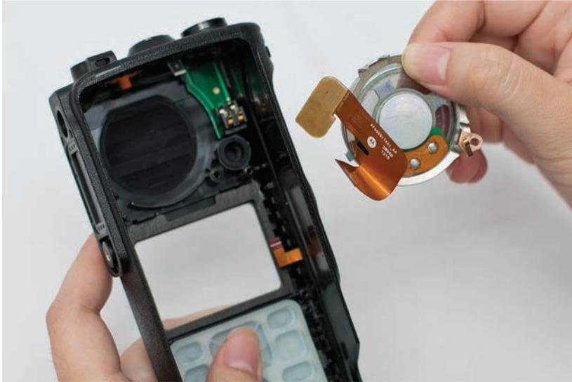
*Figure 5-22. Speaker assembly removal*
