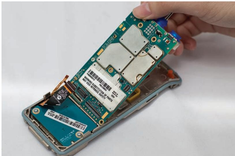
Figure 5-9. Mainboard removal
