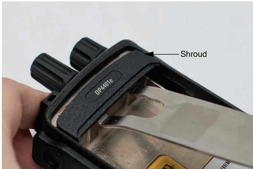
Figure 5-3. Shroud removal
