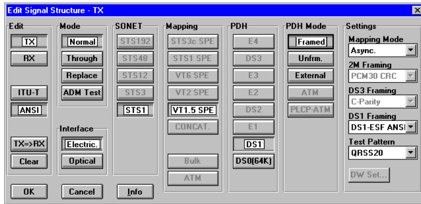
Fig. VI-2 Displaying and setting the signal structure using ANSI (Tx side) as an example
