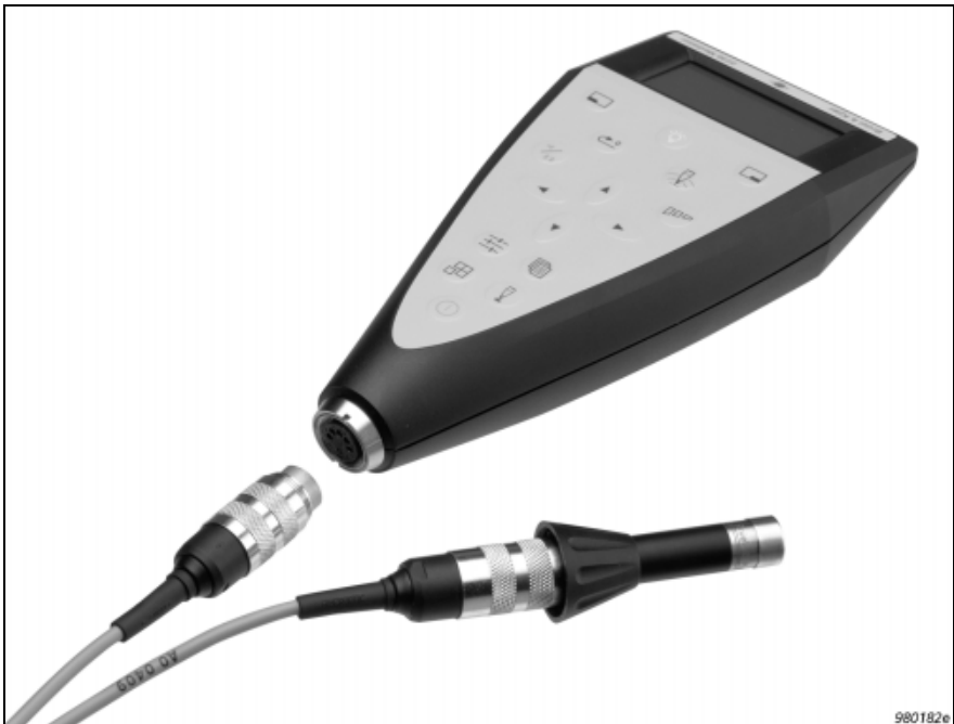
Fig.2.3 Connecting a microphone extension cable to the sound level meter
