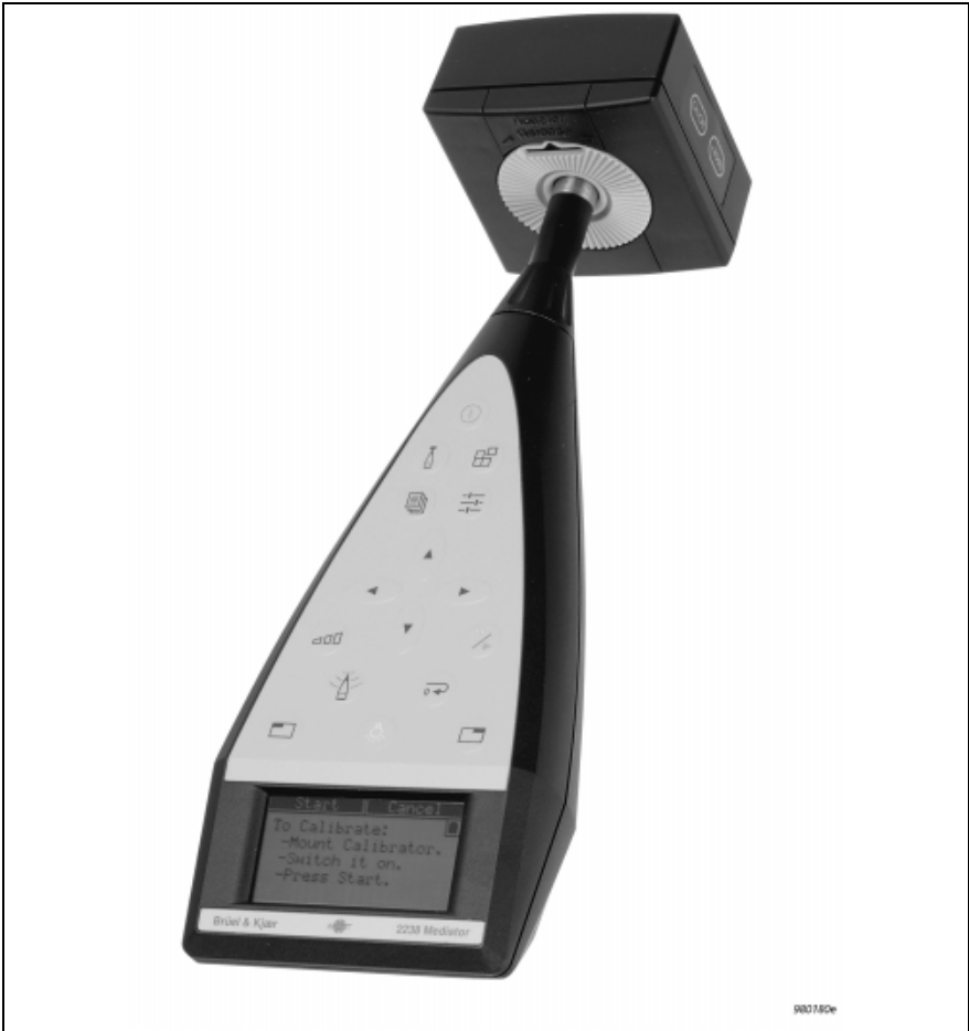
Fig.5.1 Fitting Sound Level Calibrator Type 4231 onto the Mediator. Multifunction Acoustic Calibrator Type 4226 is fitted in a similar way (see its manual)
