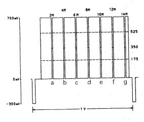
4 PAL and SECAM: 300kHz to 15MHz
