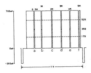
③ PAL and SECAM: 100kHz to 5MHz
