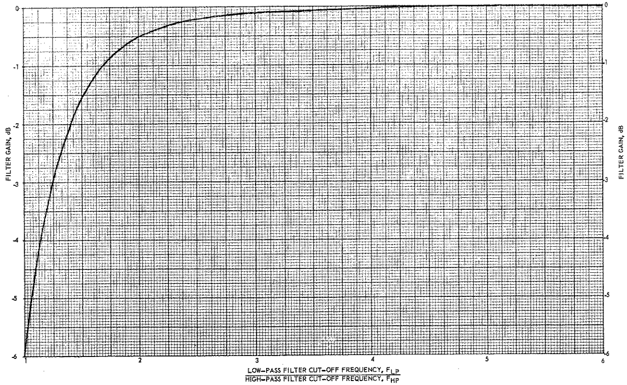
FIGURE 7 BAND-PASS FILTER GAIN VS SEPARATION OF HIGH & LOW-PASS FILTERS
