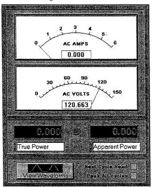
The technique used for measurements is Synchronous Sampling. This method yields maximum speed and accuracy (one-cycle measurements).
