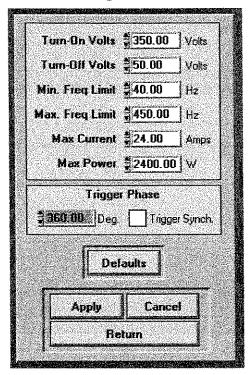
The Trig. By Voltage Transition may be programmed by the Turn-on and Turn-Off Voltages.
