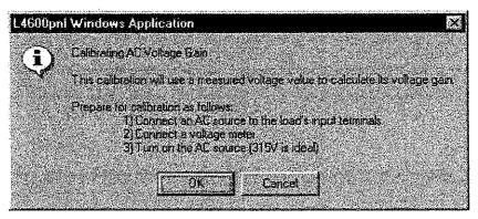
Set calibrating current and voltage to 90% of maximum rating.
