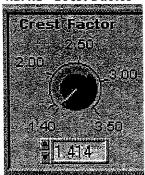
Emulates different types of load characteristics (i.e. switching supplies or other nonlinear loads) in Constant Power and Constant Current mode. Not programmable when unity power factor is selected.
