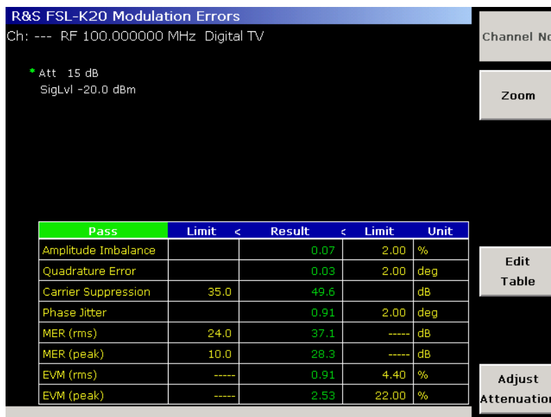
Fig. 2-55 Digital TV Modulation Errors measurement
